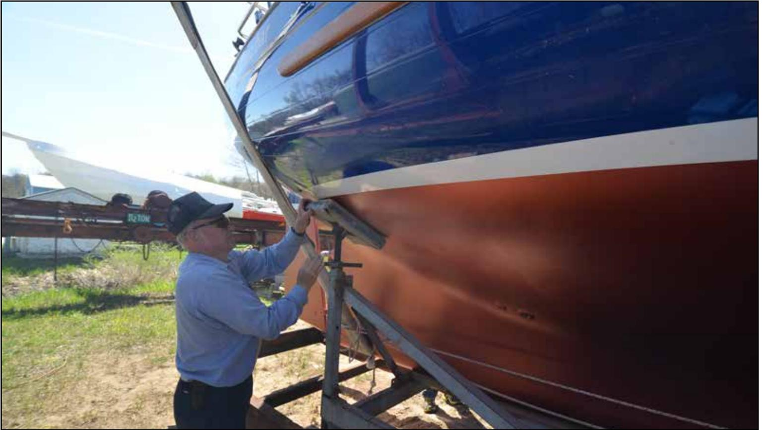
After centering , the four support pads were adjusted to the hull.
