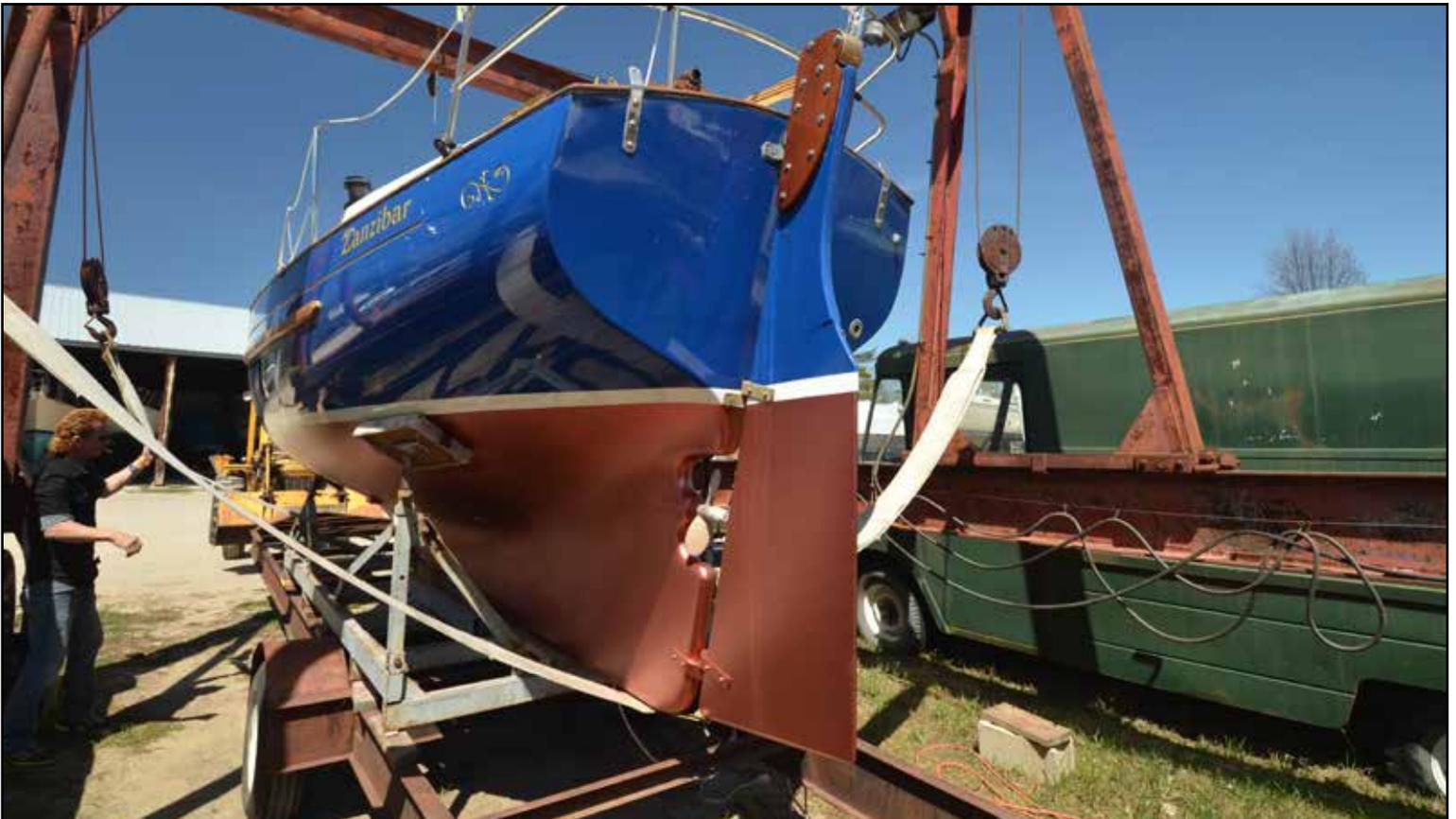
With pads adjusted to the hull, the lifting straps can be removed.
