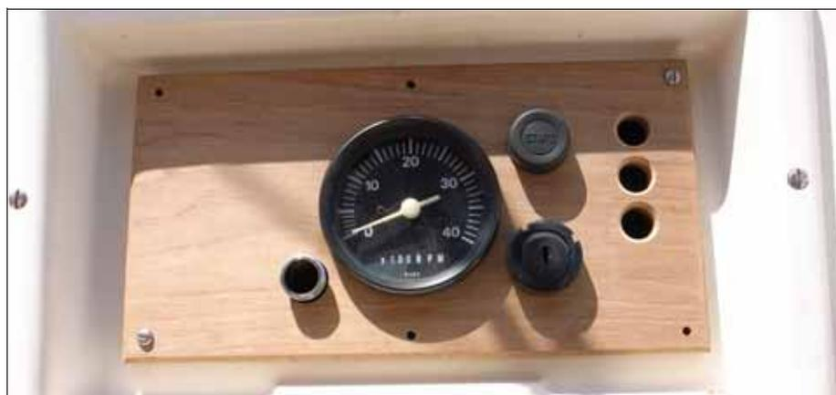
To save time, I used Epifanes Rapid Clear varnish, which can be re-coated, every 5 hours without sanding to build up five coats. I then sanded carefully with 220 grit, cleaned with a tack cloth, and applied a topcoat of high gloss Epifanes with a new brush. Finally, with the varnish dry, I could re-assemble.
