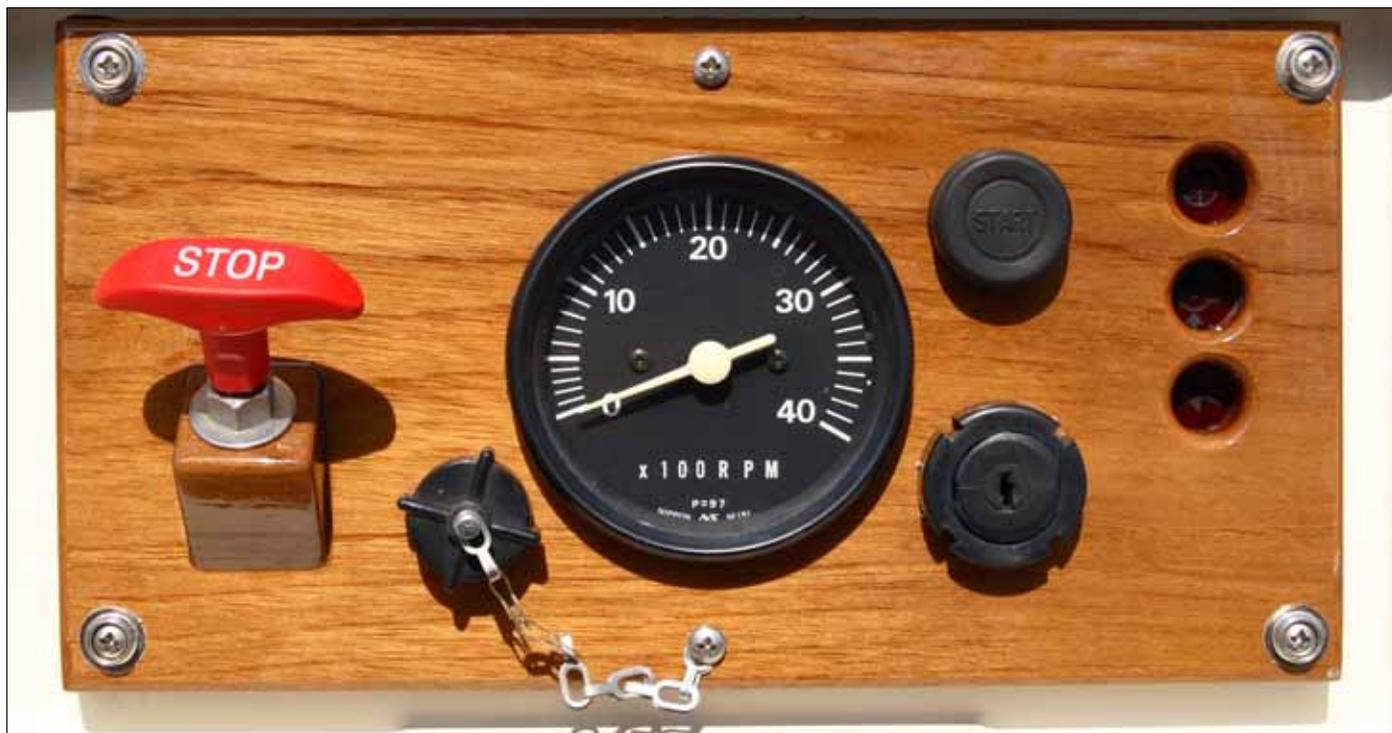
The new teak instrument panel aboard s/y **CARAWAY** includes the engine stop pull control.
