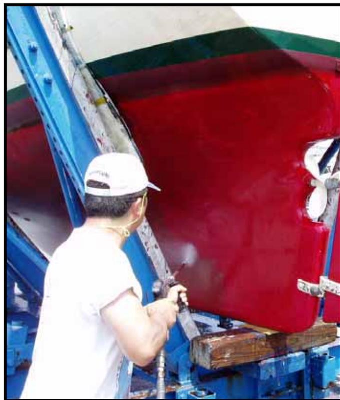
A pressure washer was used to clean the shellfish and seaweed for the hull of s/y **MARITIME**.
