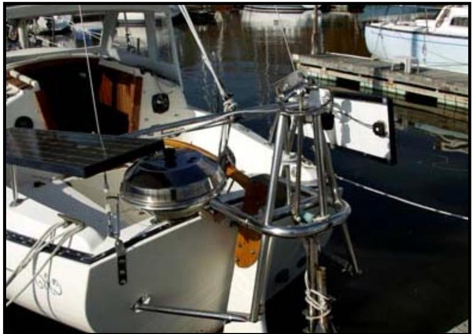
A view of PUNKER DOODLE's transom with a Monitor Windvane, propane grill, and two solar panels.
