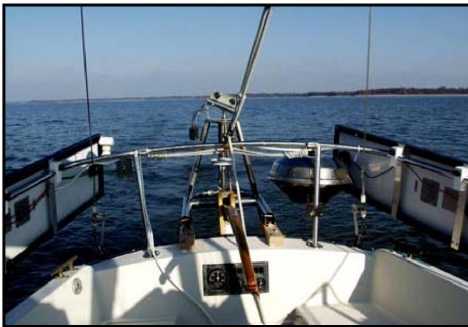
The solar panels and windvane are stowed.
