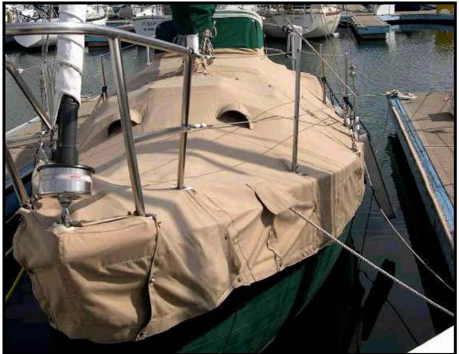
**The cover as viewed from the bow of the boat. Note how the cover goes around all hardware with flaps. Only metal is exposed.**
