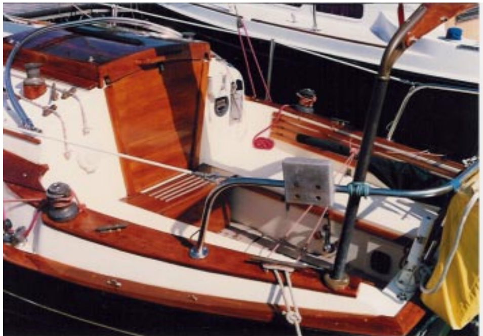
Here is a s/v SYNTHESIS II 's cockpit. Note the bridge deck and the gallows for the boom of the gaff-rig.
