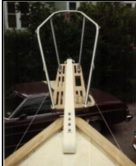
The Sitka Spruce bowsprit has a teak platform, which holds the bow pulpit and anchor roller (not shown). Part of the teak cap rail can also be seen.
