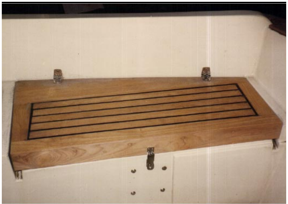
This teak hatch covers the sail locker in the cockpit. This locker also contains the manual bilge pump.
