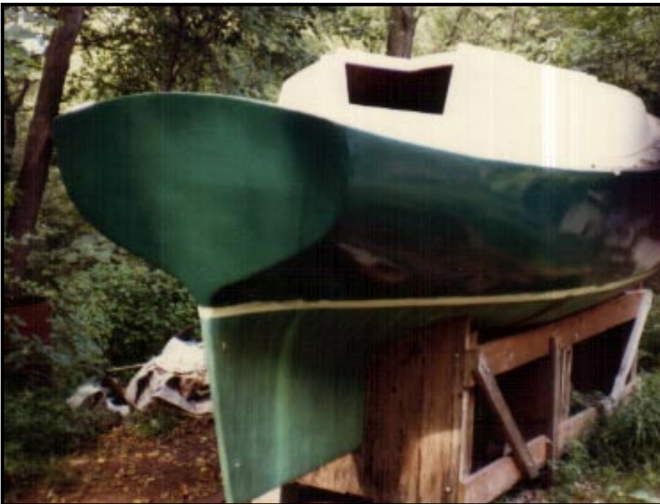
Finished Hull - This is the finished (but still empty) hull and deck after hours and hours of sanding, priming and painting.
