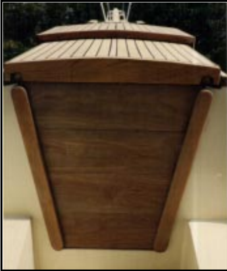
The teak hatch slides into a teak turtle hatch. Both are made of teak planking with black caulking.
