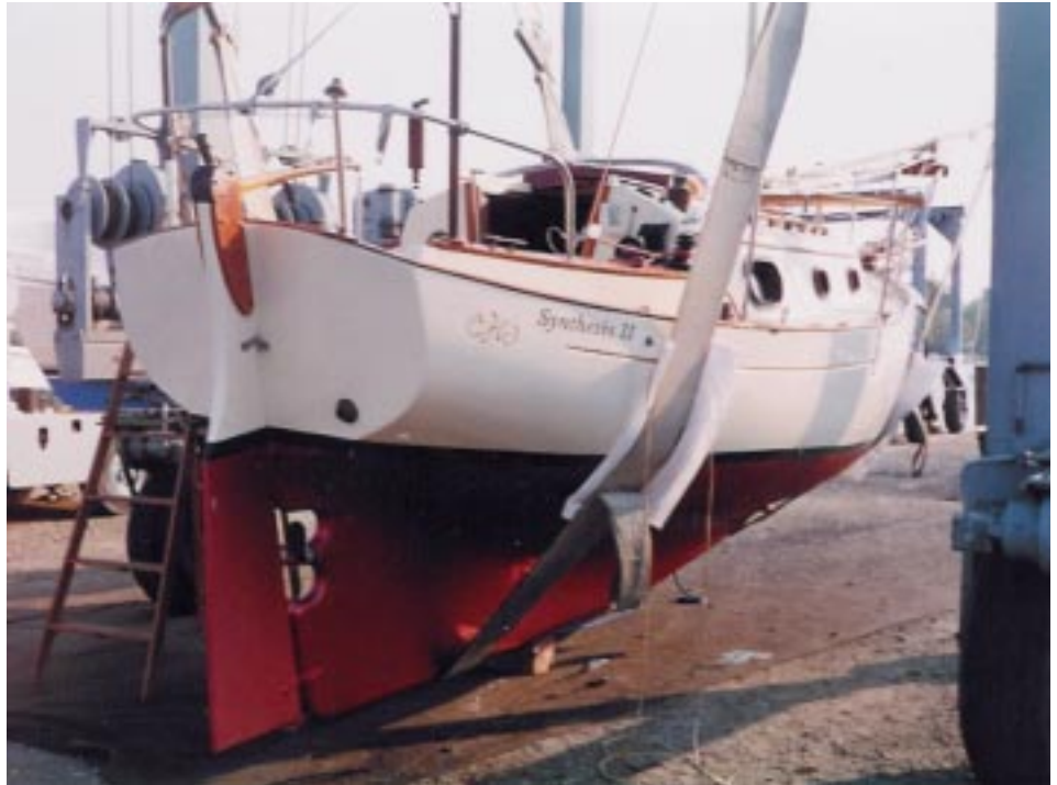
Constructed with black gel-coat, s/v SYNTHESIS II now sports a fresh coat of white paint.
