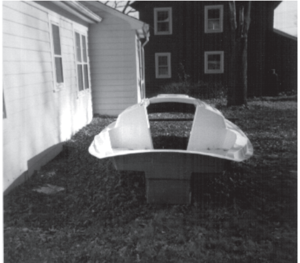
Here is the molded fiberglass deck after being shipped from California to Connecticut. I was glad to let Pacific Seacraft help speed up my project!
