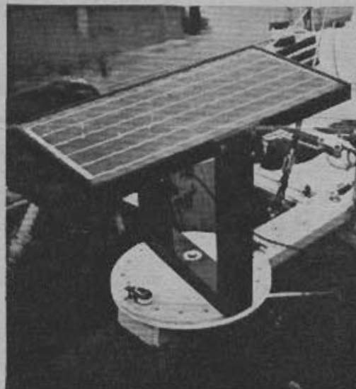
Above is John's solar generator that can follow the sun just about anywhere.
