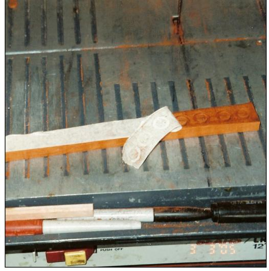
3. Adding tape to control plugs while cutting with band saw. **Photo: Bob Collier** © **2014**
