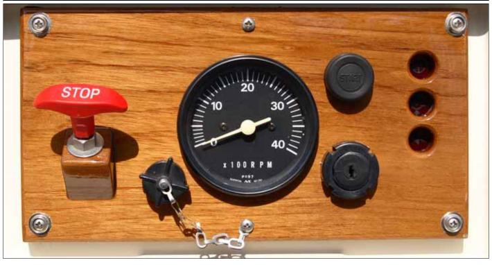
The new teak instrument panel aboard s/y CARAWAY includes the engine stop pull control.
