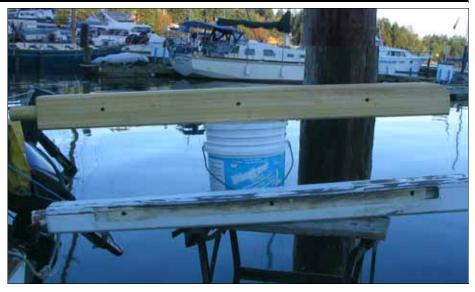
Here is the old bow sprit and the new replacement. The new one has a larger cross-section than the factory original allowing the platform holes to be drilled closer to center. *Photo: James Boles* © 2006
