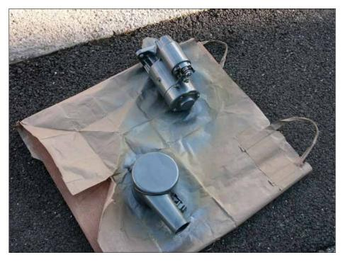
The air cleaner housing and starter motor receive a fresh coat of paint. *Photo: Benjy* © 2006
