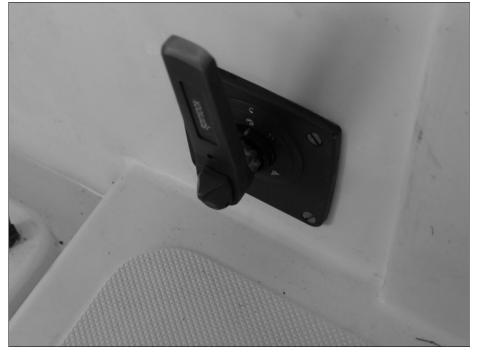
The new shift and throttle lever combined shifting and throttle into one. *Photo: Benjy* © 2006
