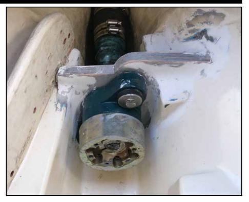
After considerable trial and error, the thrust fitting was installed. *Photo: Benjy* © 2006
