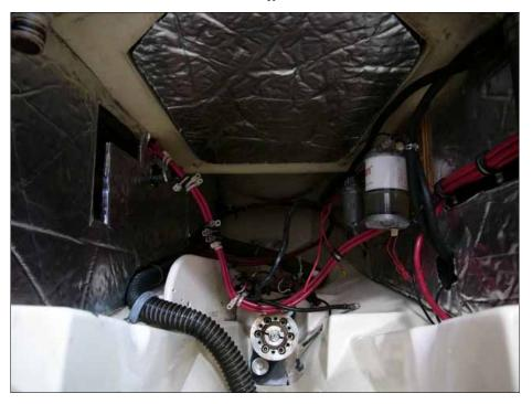
A layer of sound proofing was also added to the engine hatch. Also, notice the new gel coat finish in the engine bed. *Photo: Benjy* © 2006
