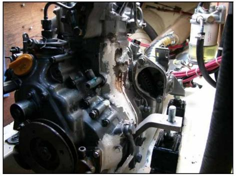
The first step was to free the engine from the engine compartment. *Photo: Benjy* © 2006
