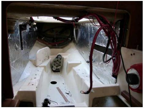
With the engine out, sound proofing was added to the engine compartment. *Photo: Benjy* © 2006
