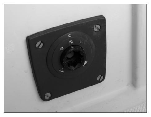
Unlike the original two lever arrangement, the Spinlock lever can be removed when not needed. This prevents mainsheet complications. *Photo: Benjy* © 2006
