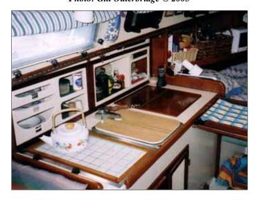
Interior showing the galley and custom stowage. The tiled stove top lifts off and sets on the folding table to left and is useful for hot pans etc..
