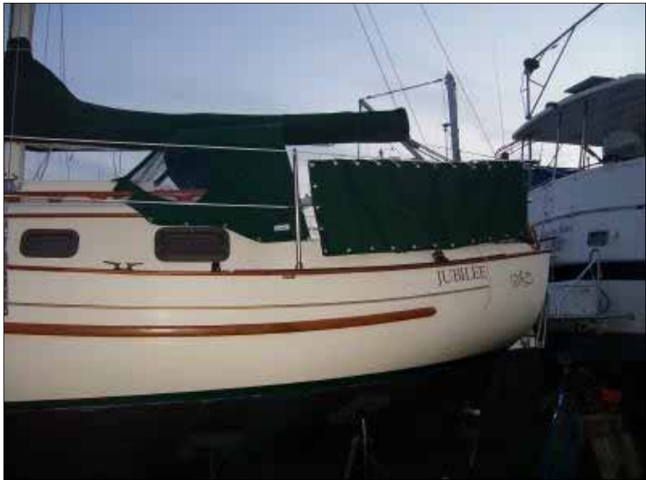
A new dodger, weather cloths, and sail cover were installed. Photo: Frank Durant © 2007
