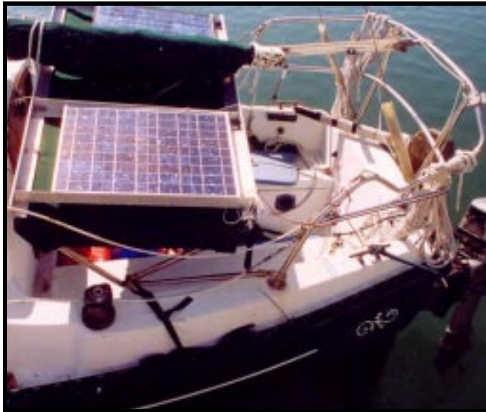
The rigging and aft pulpit were also destroyed.
