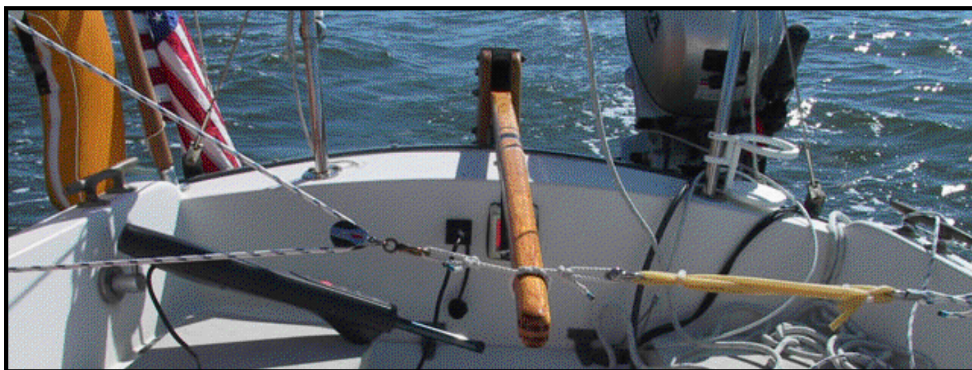
These two photos show the tiller attachment and pulley arrangement for a self-steering for a Flicka.
