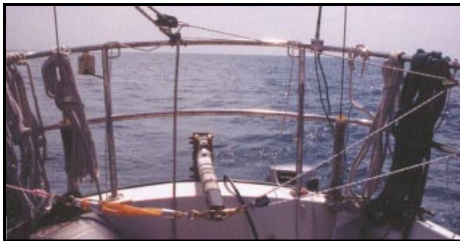
s/v Solar Wind with Sheet-To-Tiller steering using the Mainsheet
