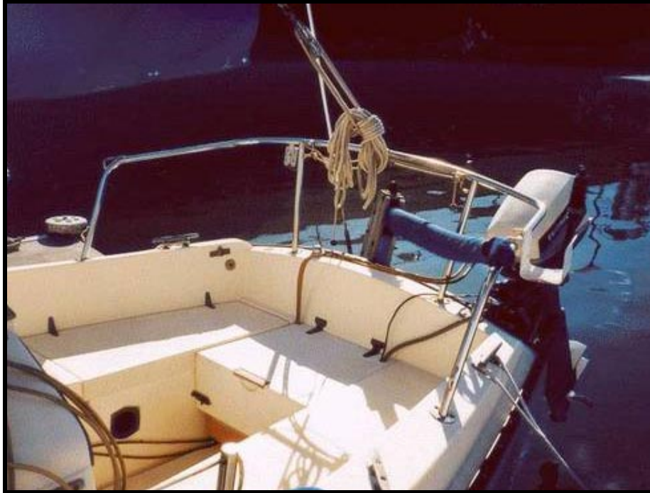
A typical placement of an outboard engine on the port side of the transom. Note the fuel tank storage in the cockpit.
