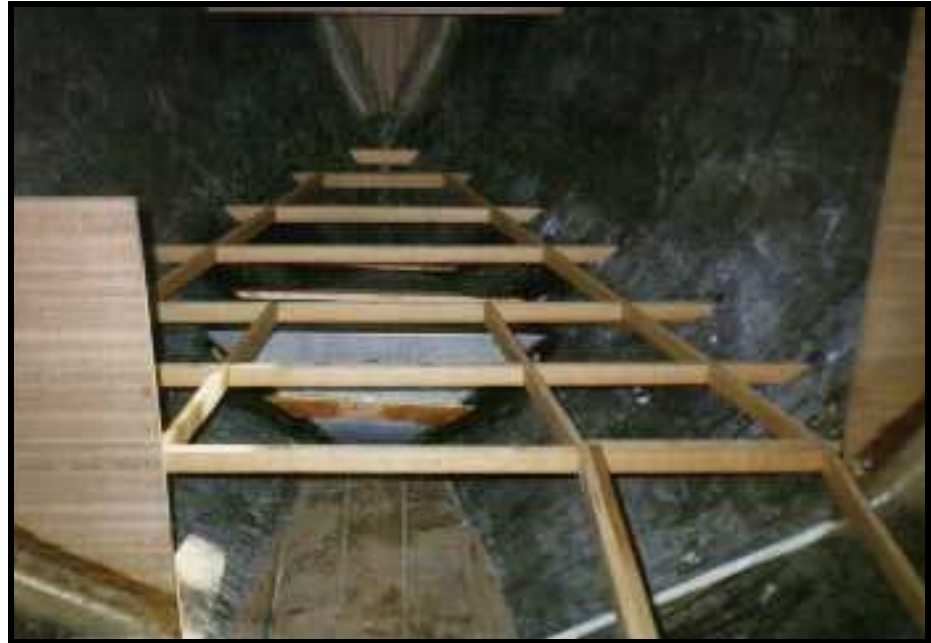
Forward Berth Framing – This is the roughed-in framing for the v-berth showing the partial bulkheads on either side, the bow tank and the forepeak bulkhead.
