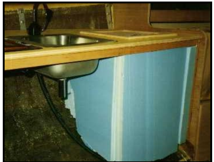
Unfinished Galley – This is the rough galley lay out with the alcohol stove, the sink and the icebox
