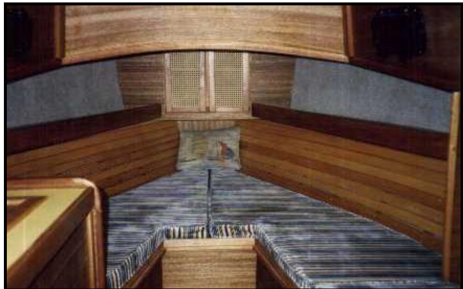
Finished Forward Cabin – This picture shows the completed forward cabin, complete with the maple ceiling strips.
