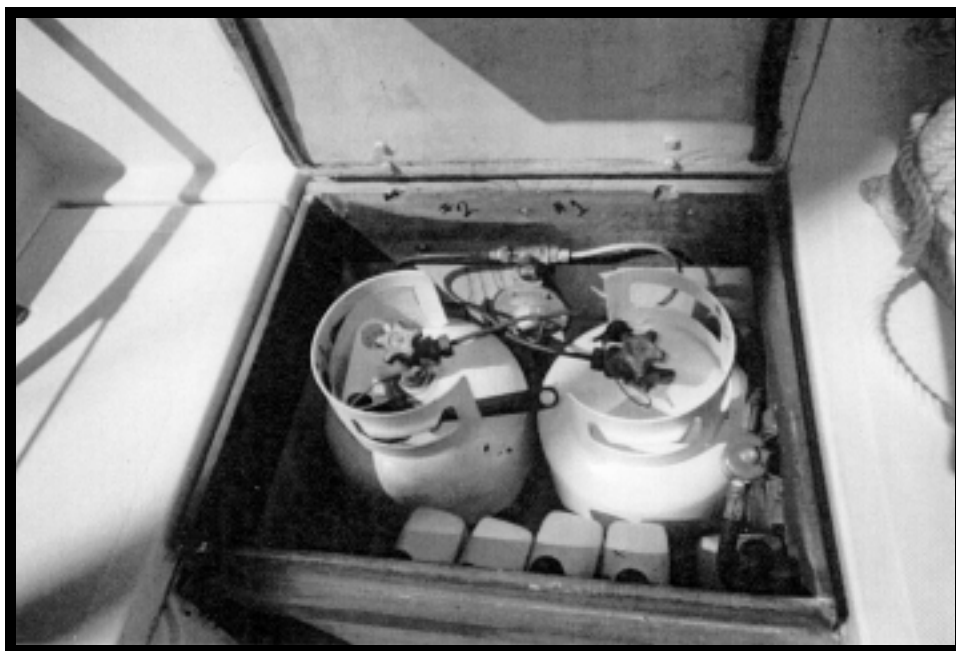
The propane storage box located in the aft cockpit of TAN BARQUE (Pacific Seacraft Flicka # 277)
