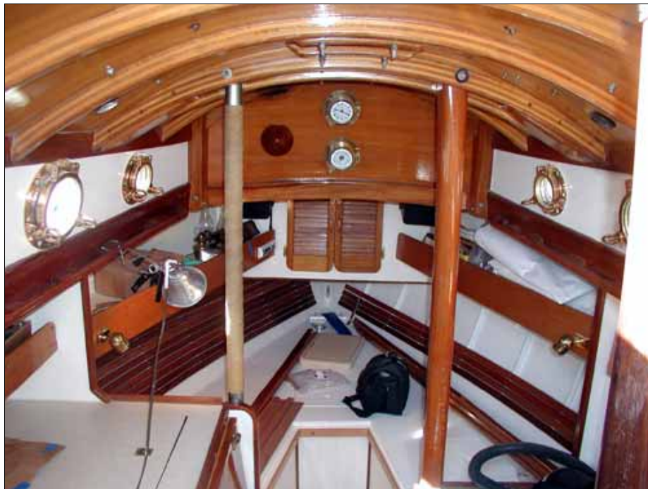
Rudder post and scrap mahogany poles were used in place of hanging knees in original build. Provided great handholds at sea.
