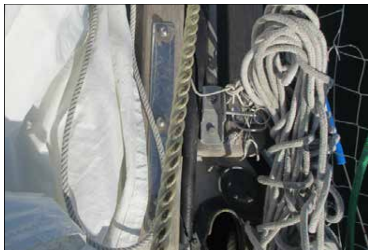
Day 2. Anchor rode chafe from something on the sea floor. Photo: Josh Wheeler © 2018
