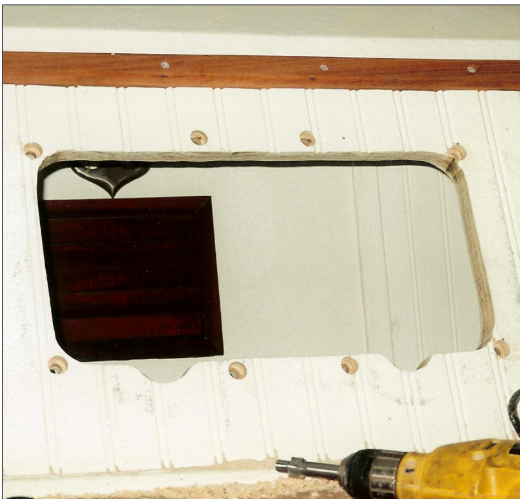
A special drill bit cuts the holes and creates the recess as well. Photo: Bob Collier © 2016
