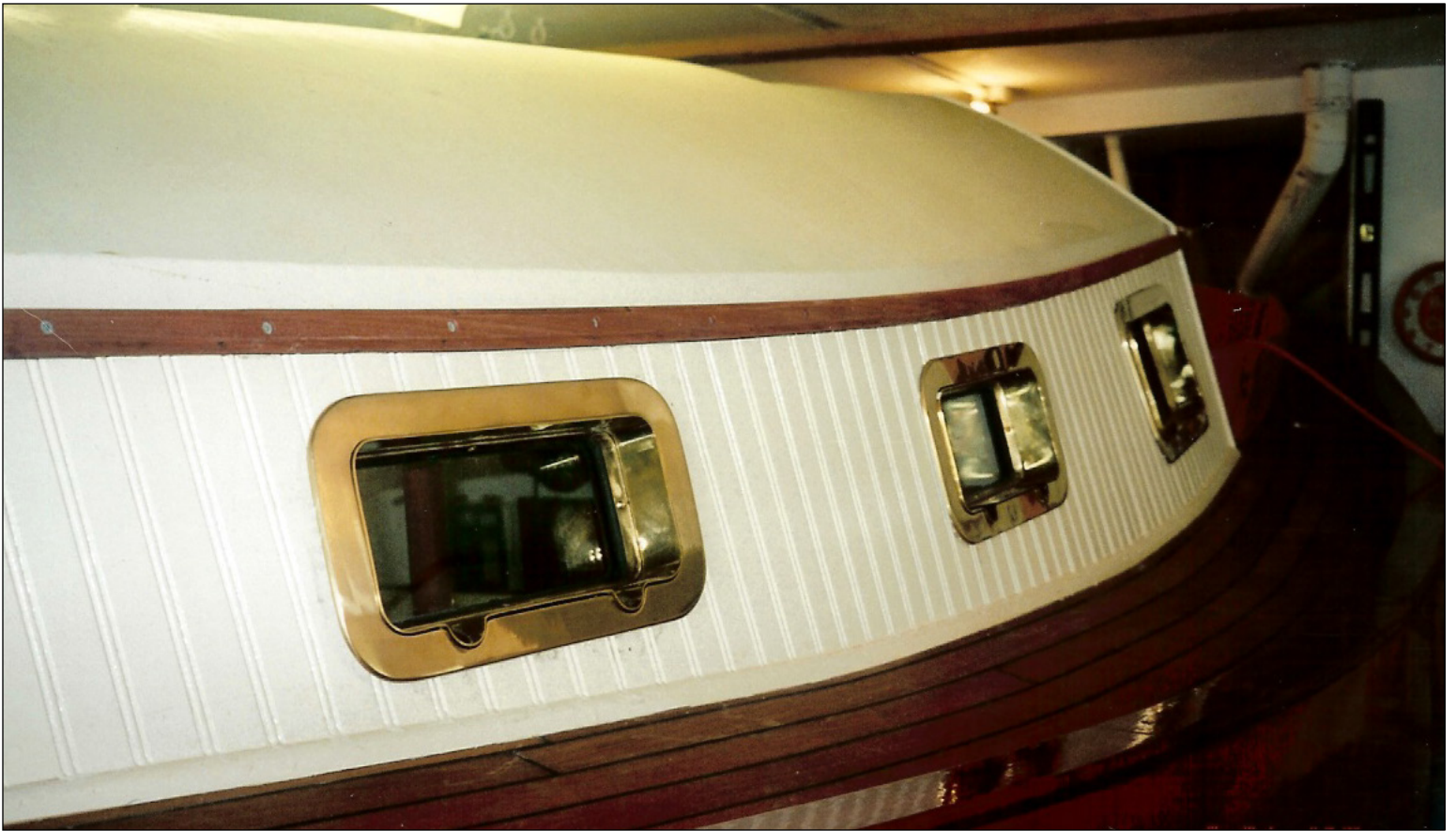
Three Newfound Metals port lights in place on the port side of s/y RED RASCAL . Photo: Bob Collier © 2016
