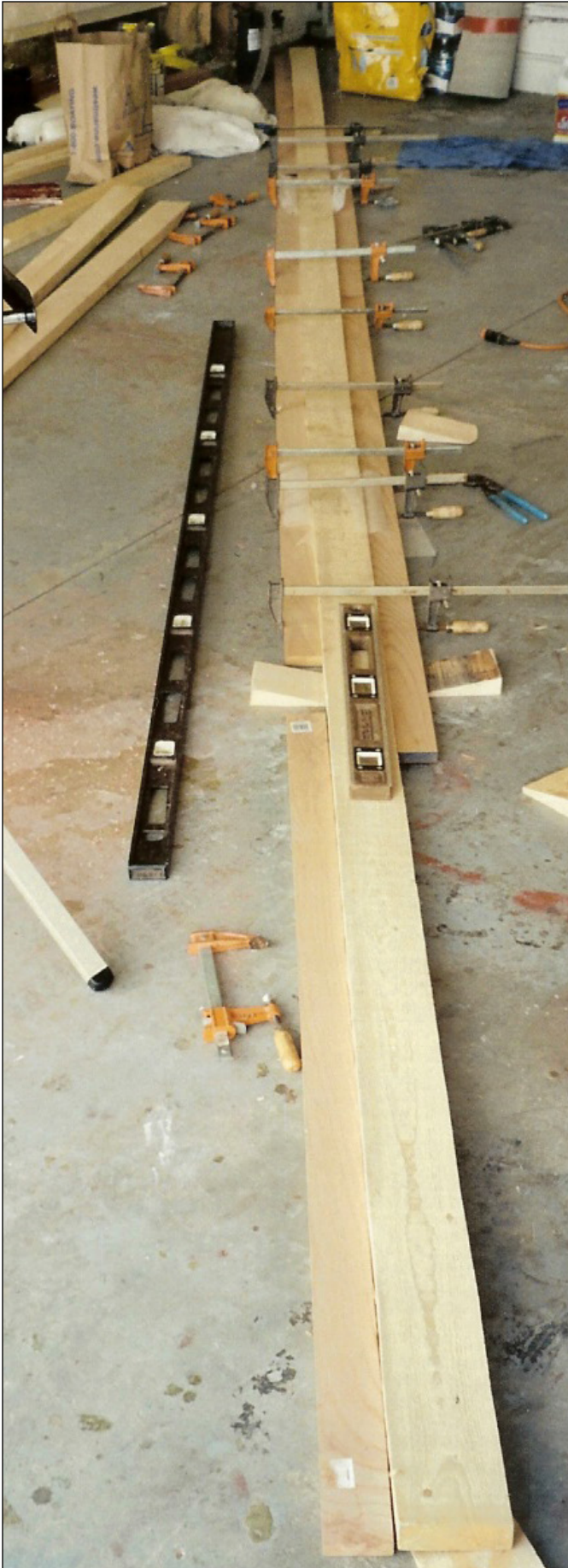
Scarfing the mast sections. Photo: Bob Collier © 2016
