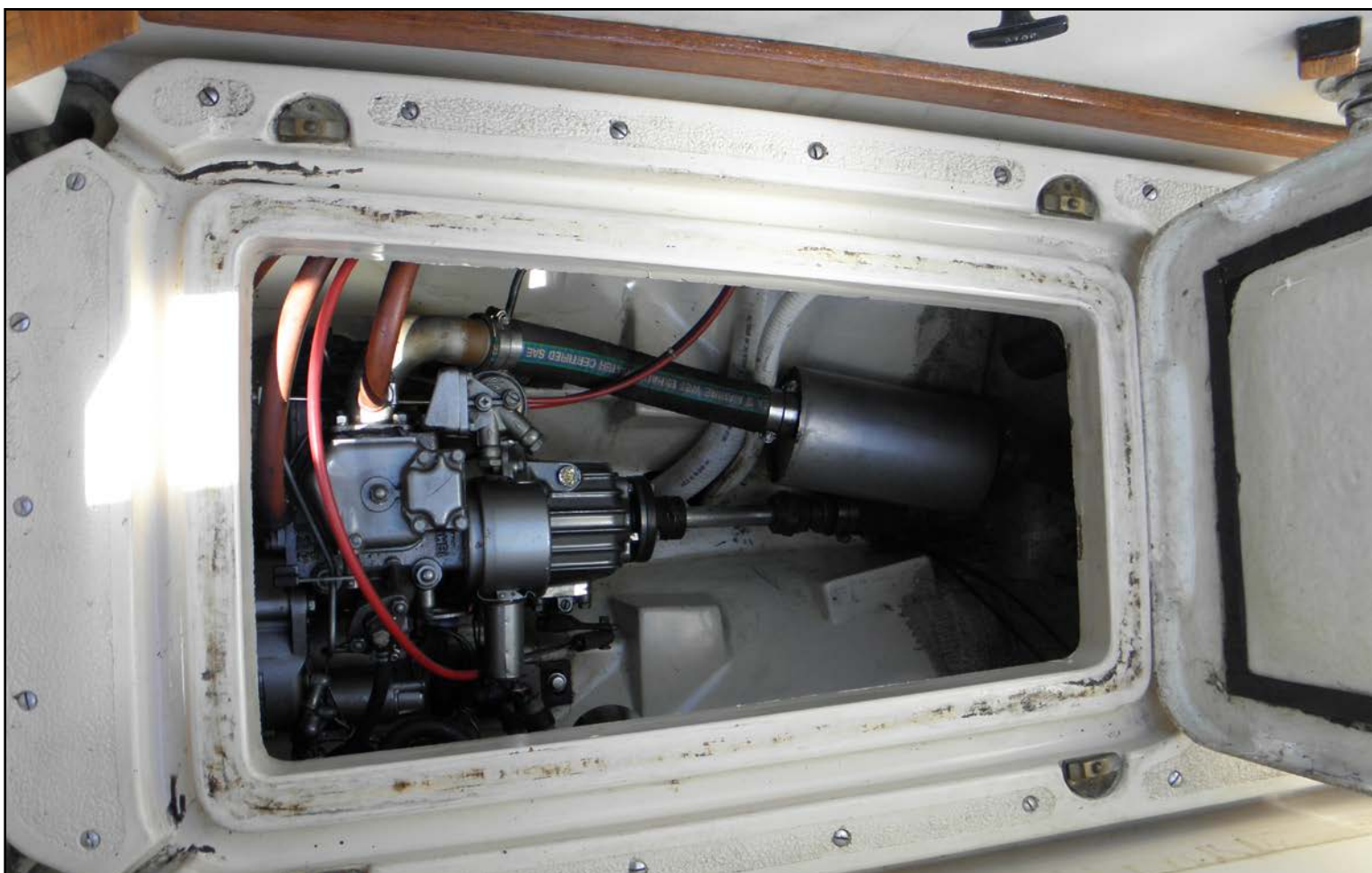
The Yanmar 1GM diesel inboard engine. The hinged cover is a nice feature that is missing on the newer hulls. Photo: Bob Borgilt © 2015
