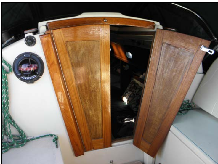
A set of folding doors replace the hatchboards aboard s/y ESCAPE . Photo: Bob Borgilt © 2015
