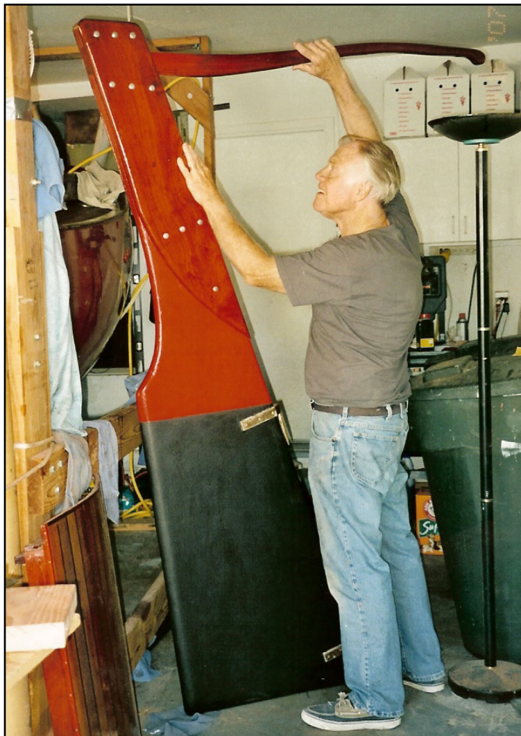
Upper Left: The pieces of the rudder ready for woodworking.
