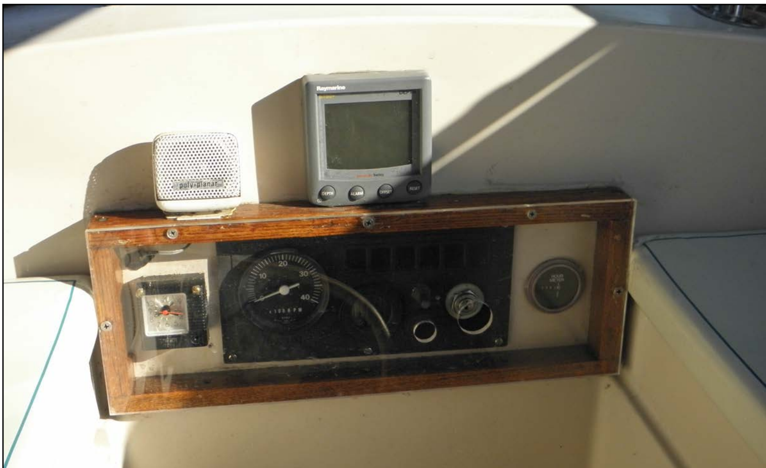
Engine control panel with a clock (tidal area), hour meter, speaker, and depth finder. Photo: Bob Borgilt © 2015
