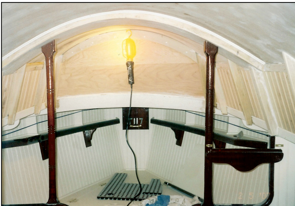
Upper Left: Installing the forward wall of the cabin.
