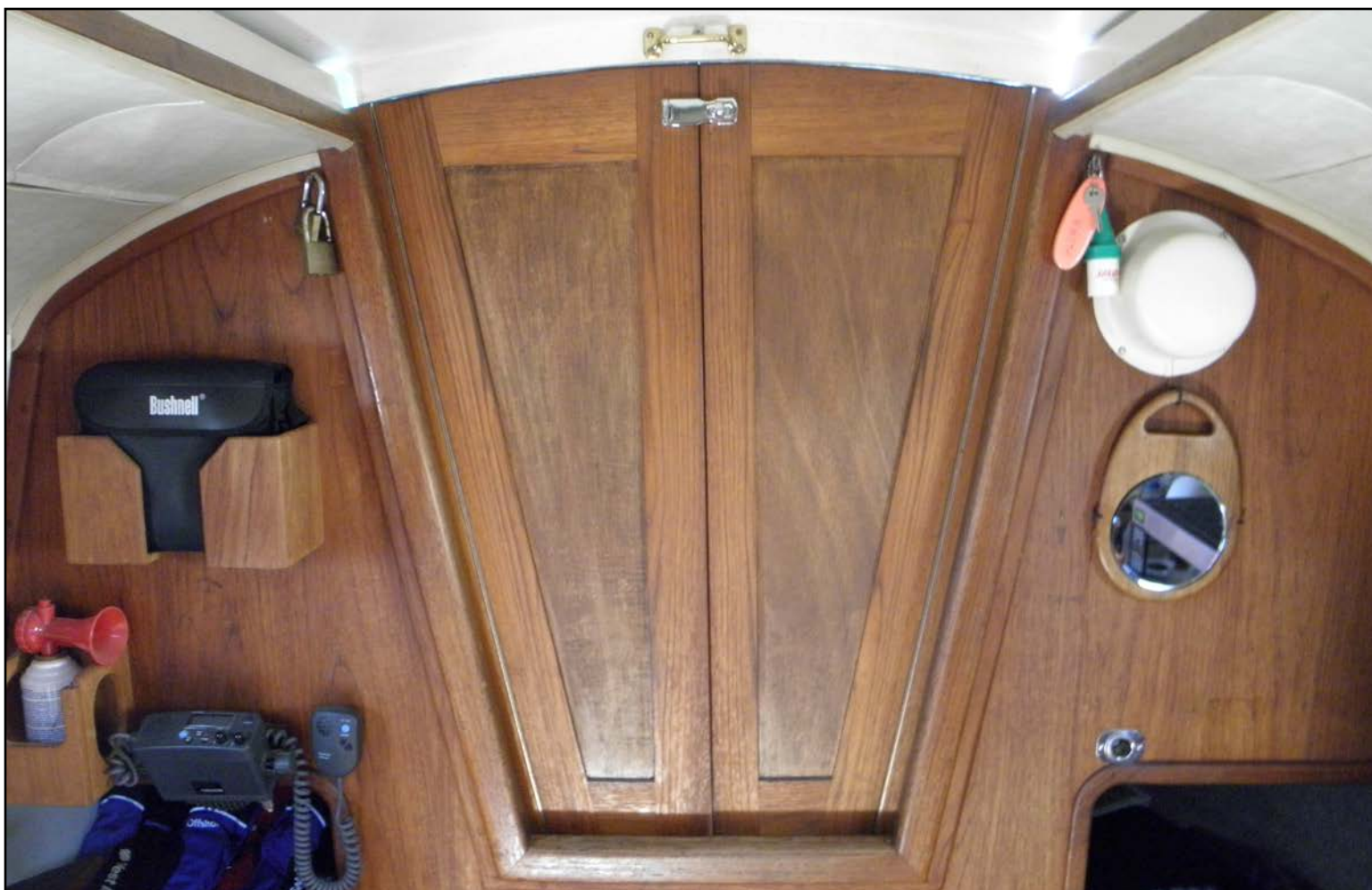
Folding companionway doors of s/y ESCAPE viewed from the cabin. Photo: Bob Borgilt © 2015
