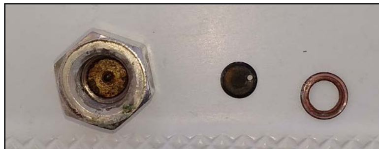
The joker valve nut, diaphragm, and washer, Photo: Roger Weinheimer © 2015
