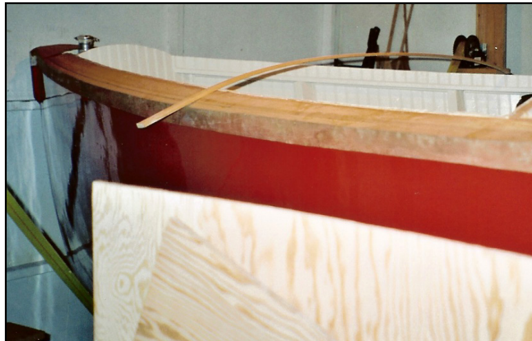
A batten was used to determine the correct deck camber. Photo: Bob Collier © 2015
