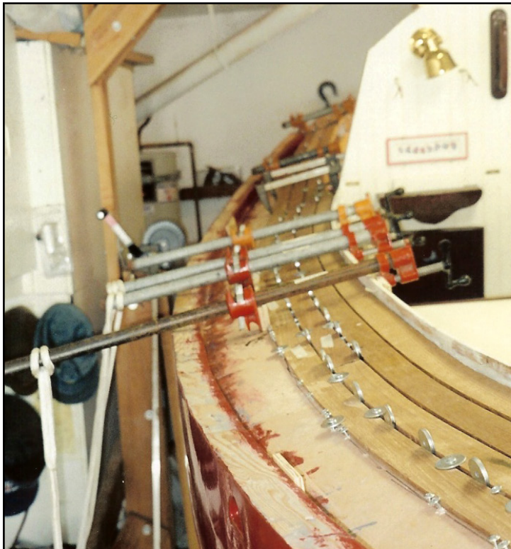
Above: Clamps and washer were used to place the planks. Photo: Bob Collier © 2015
