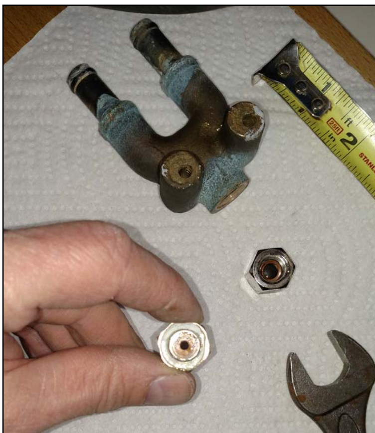
A 7 mm wrench is needed for removal. Photo: Roger Weinheimer © 2015
