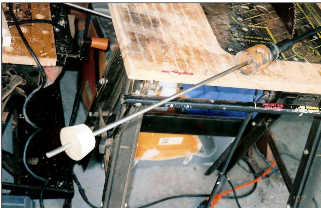
A drill extension, hole-saw, rod, and "cork" was used to drill the propeller shaft. Photo: Bob Collier © 2015
