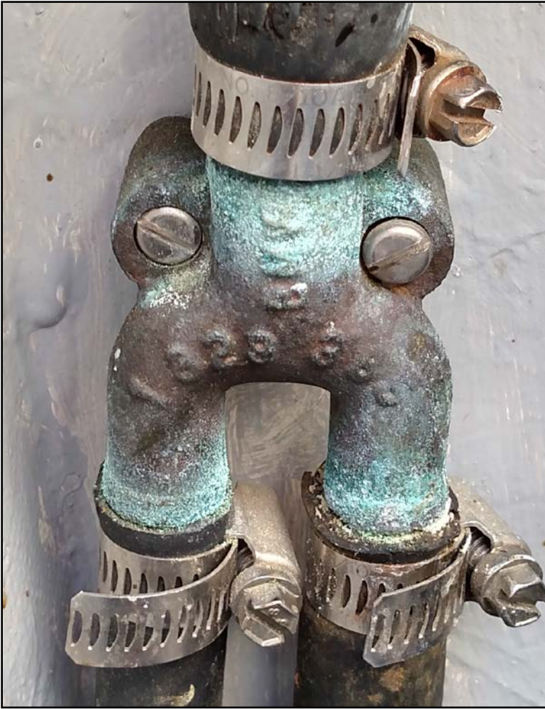
The joker valve is underneath the top hose. Photo: Roger Weinheimer © 2015
