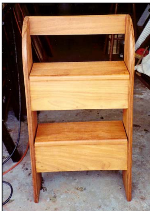
The diagram shows the basic construction of the steps. There are multiple screws and glue holding the base of the steps. The cabin steps also provide additional storage. I've put non-skid tape on the treads and hinges inside the lid. Photo: Bob Collier © 2015
