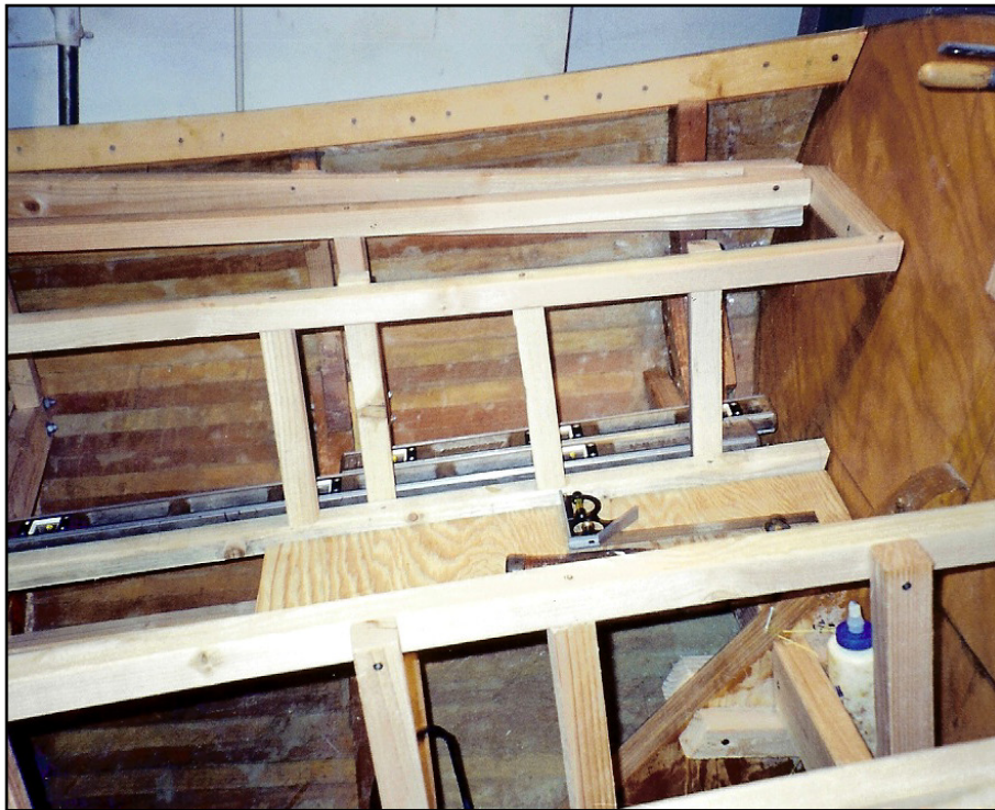
Framing the cockpit of s/y RED RASCAL . Photo: Bob Collier © 2015
