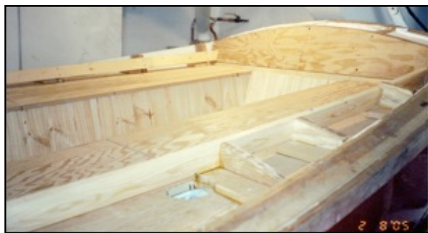
Note the coaming construction. Photo: Bob Collier © 2015
