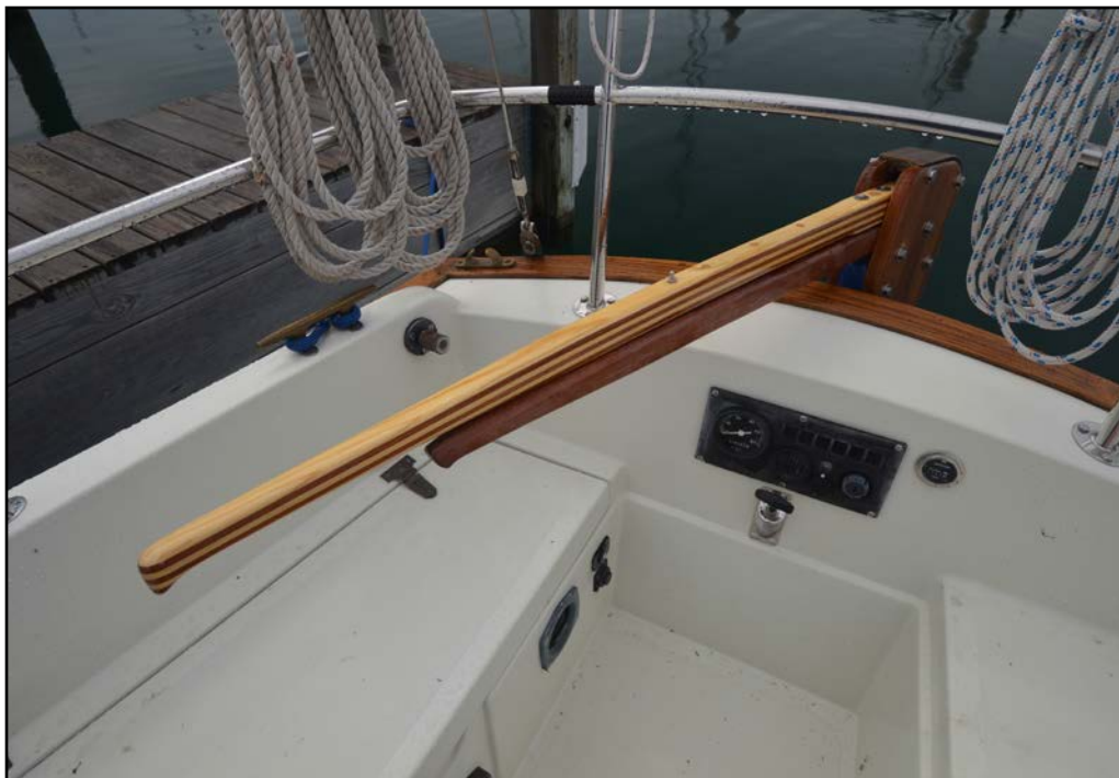
The old tiller is resting on top of the emergency tiller. The primary reason for being shorter is that the mahogany piece was available at home.
