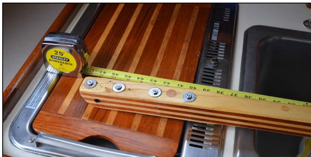
Four bolts were added to the old tiller to strengthen the laminations. While not bristol, this tiller is quite serviceable as an emergency backup.
