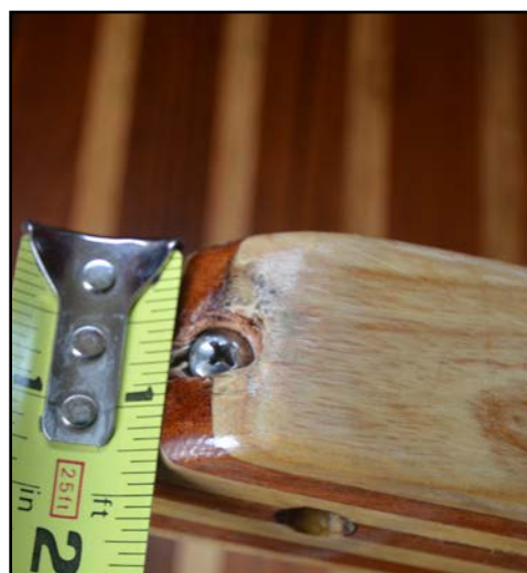
The width of the delaminated tiller is 1.5 inches. The height is 2.0 inches. Rudder Craft recommends confirming these dimensions before ordering.
