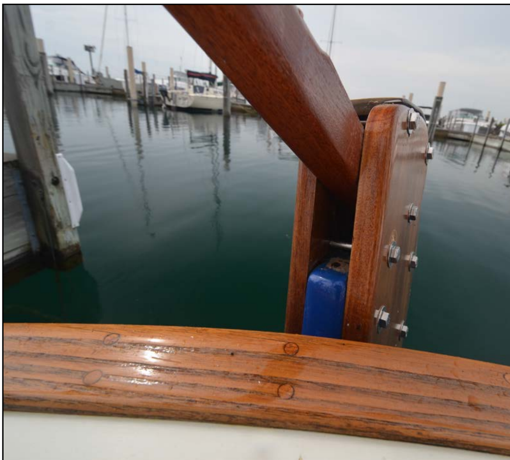
Note the rudder bolt that acts as a fulcrum. Not all Flickas have this bolt. Photo: Tom Davison © 2015
