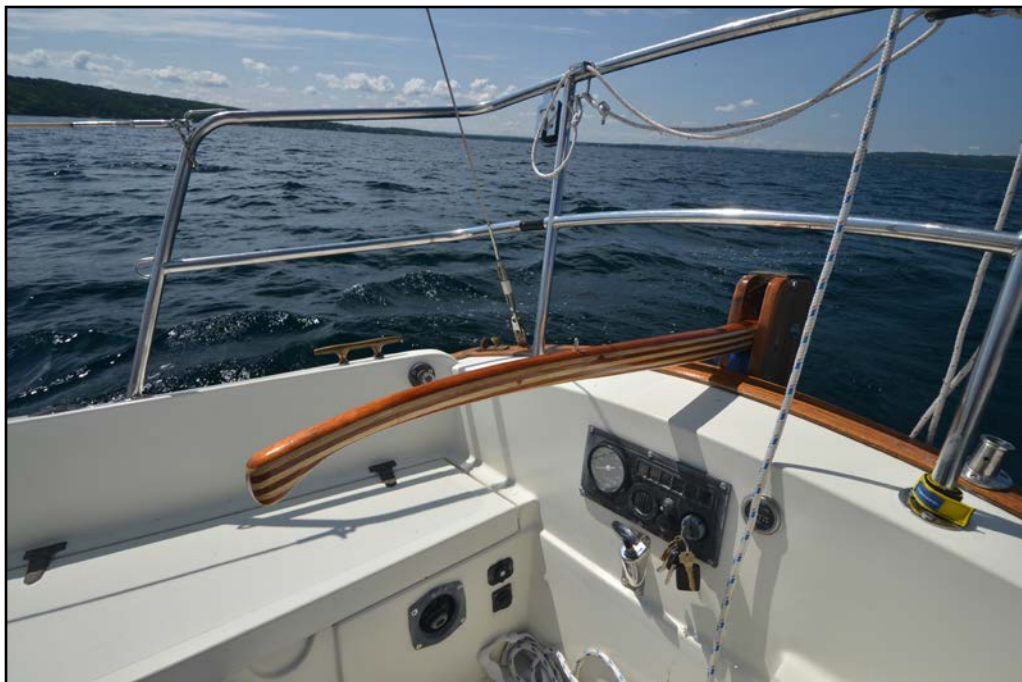
The new tiller aboard s/y ZANZIBAR is shorter than some and almost completely straight, extending just forward of the stern rails. Photo: Tom Davison © 2015
