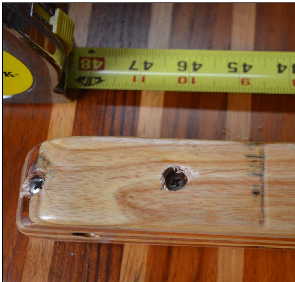
Note the indentation caused by the rudder bolt on the tiller.
