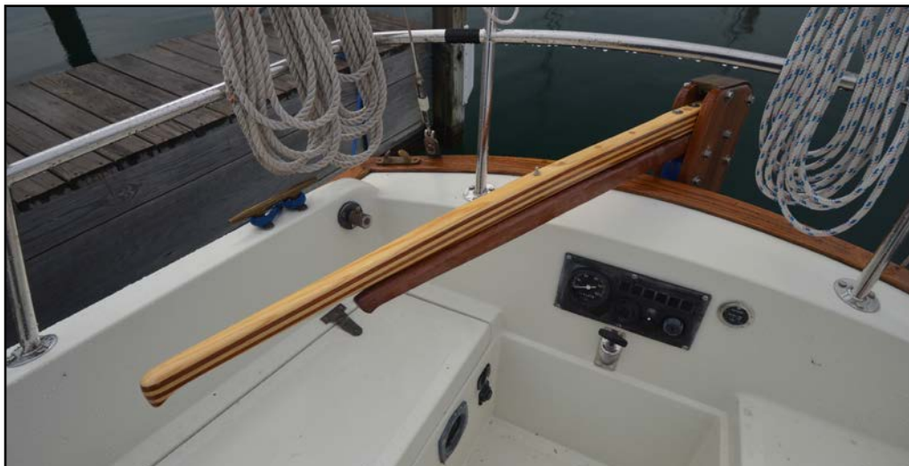
The old tiller is resting on top of the temporary emergency tiller. The primary reason for being shorter is that the mahogany piece was available at home.
