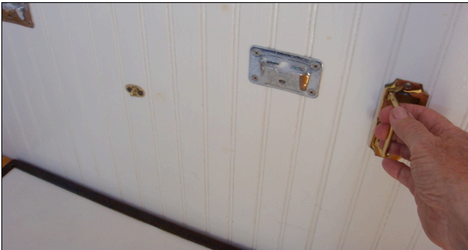
The back of the dinette is removable and can be used to create a second sea berth on the port side. Photo: Bob Collier © 2014
