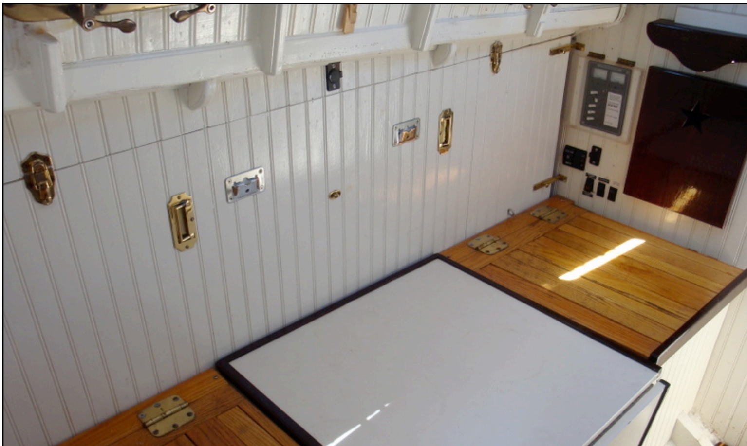
The table fills in the dinette for a sea berth. Photo: Bob Collier © 2014
