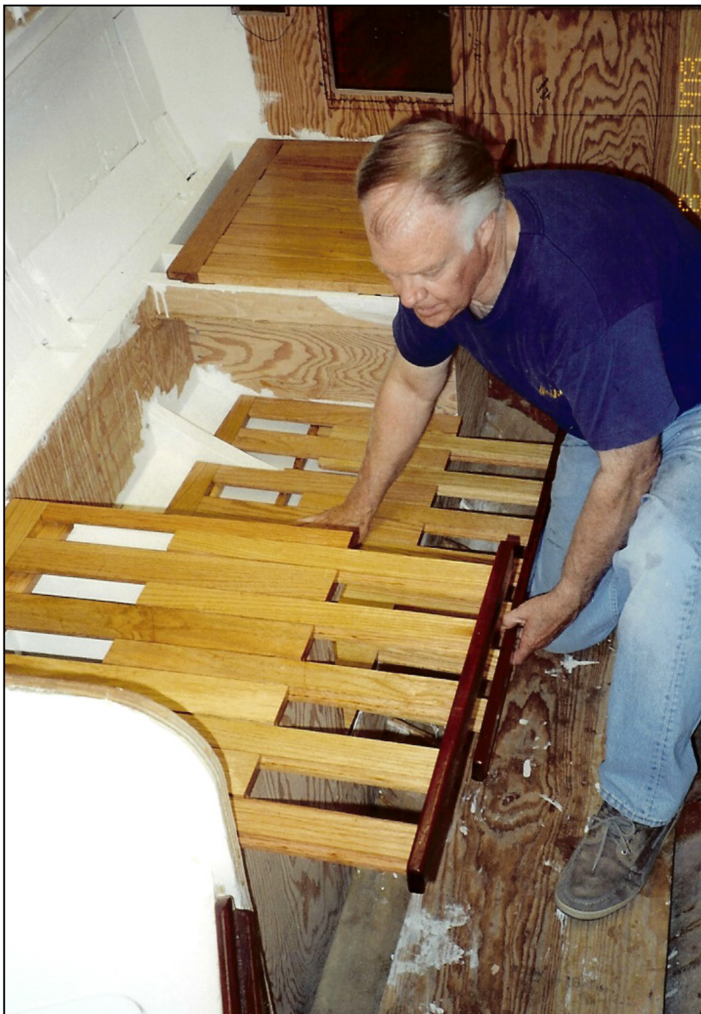
Construction of the convertible dinette and sea berths. Photo: Bob Collier © 2014
