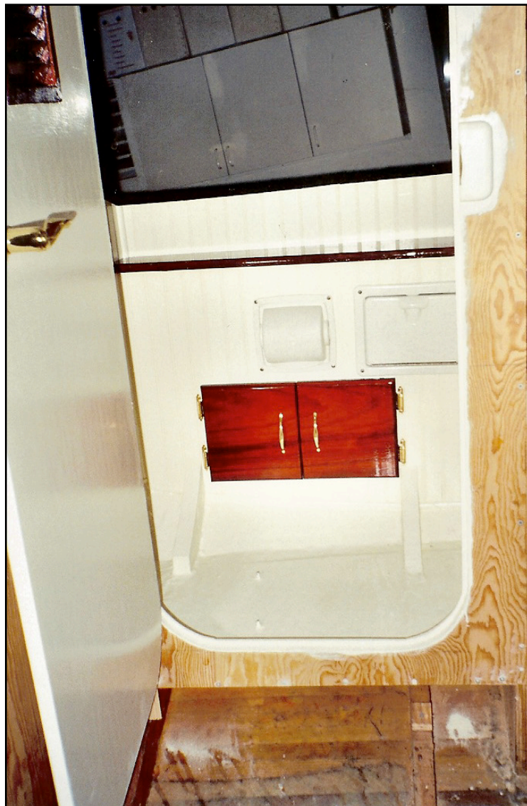
Photo 5: Head compartment painted and ready for the head. Photo: Bob Collier © 2014
