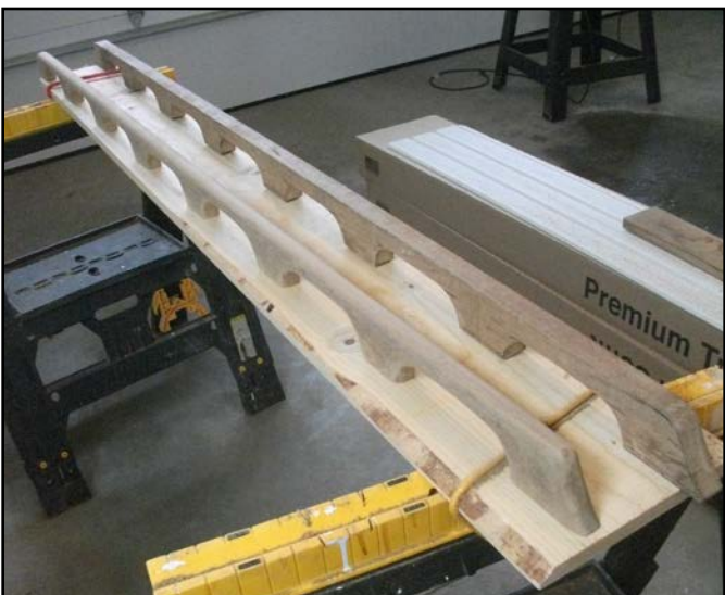
Handrails cut out with a jig saw. Photo: Randy Richardson© 2014
