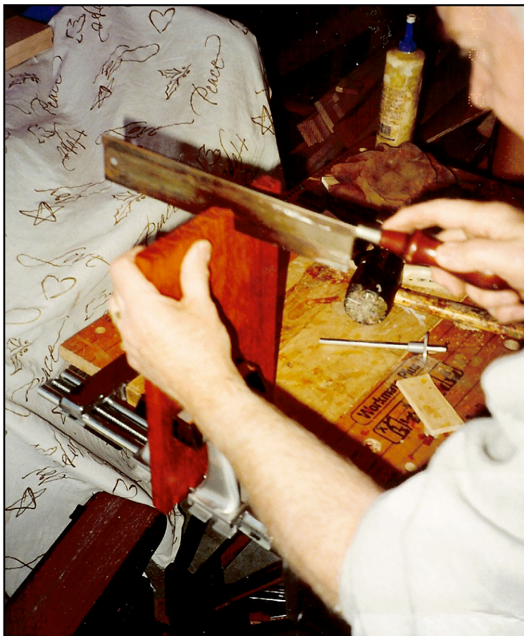
Photo 10: Cutting the dovetail joints for the drawers. Photo: Bob Collier © 2014
