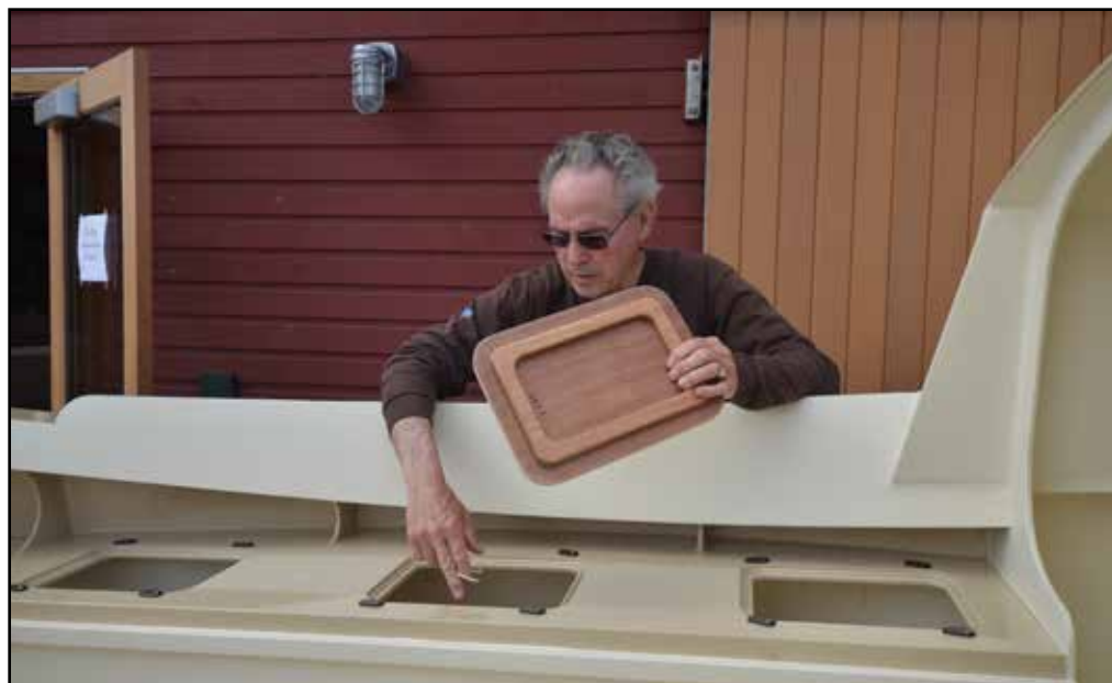
Three watertight hatches create positive floatation for the Scamp. Photo: Tom Davison © 2014
