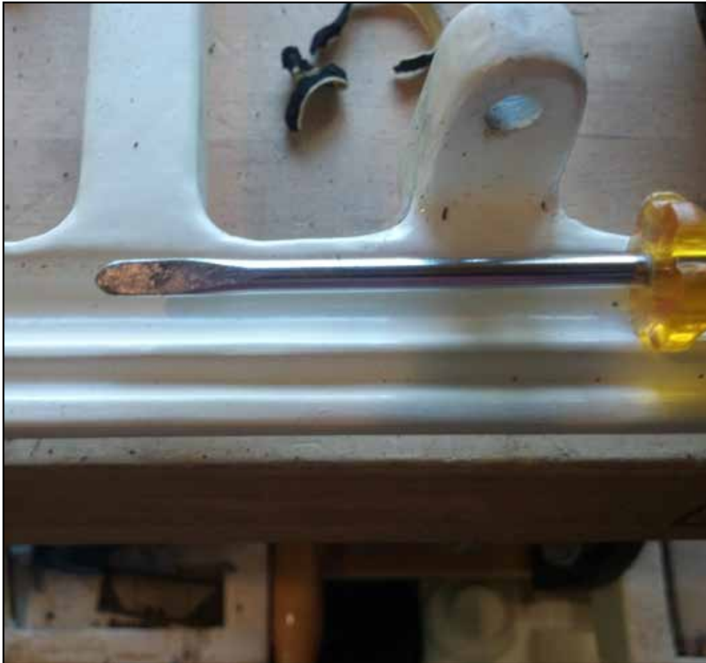
A screwdriver was modified to remove the gasket from the Bomar hatch.
