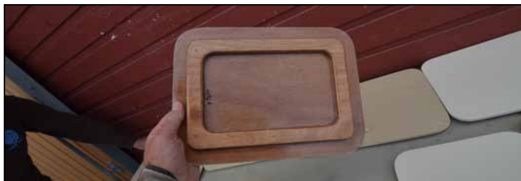
Three watertight hatches also protect the items stored under the seats. Photo: Bill Hogan © 2014
