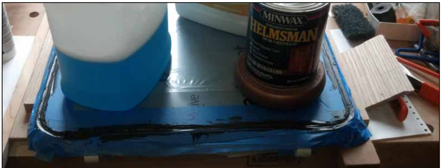
The new masked lens is embedded in the new adhesive and weighed down to set. Now, just waiting for it to cure. Photo: Daryl Clark © 2014
