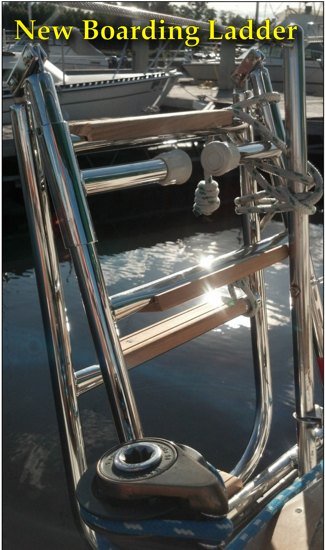
A Mystic stainless steel boarding ladder was installed on the port side of my Flicka. Photo: Daryl Clark © 2014
