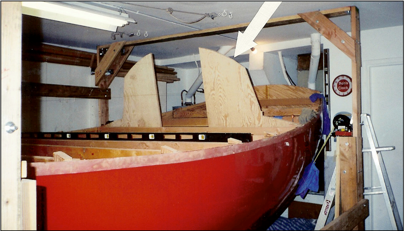
Photo # 8: With RED RASCAL turned over, it was time to build a cradle. The first bulkhead's angle was checked as well. Photo: Bob Collier © 2014
