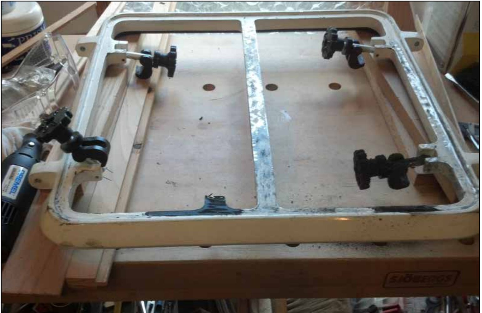
Nearly done with the removal of the old adhesive from the hatch frame. Photo: Daryl Clark © 2014
