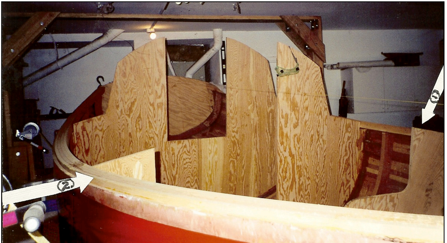
Photo # 9: A 3" x 4" beam runs stem to stern. It adds rigidity and a surface for the deck to rest upon. Photo: Bob Collier © 2014
