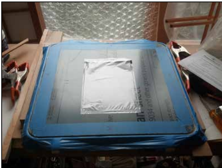
Masking completed on the outside of the lens. Photo: Daryl Clark © 2014
