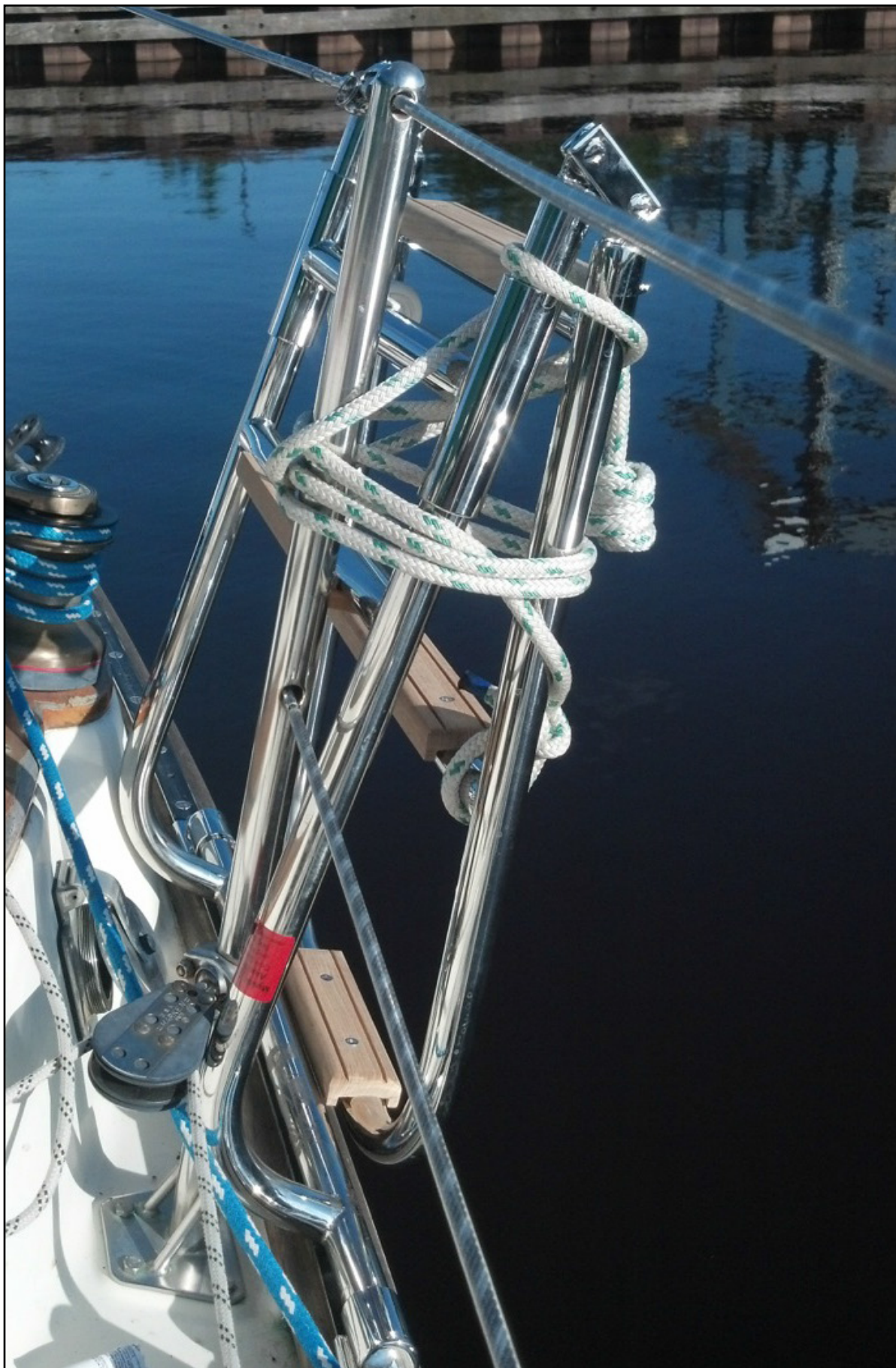
The stainless steel ladder folds up against the life lines and is quickly ready for use.
