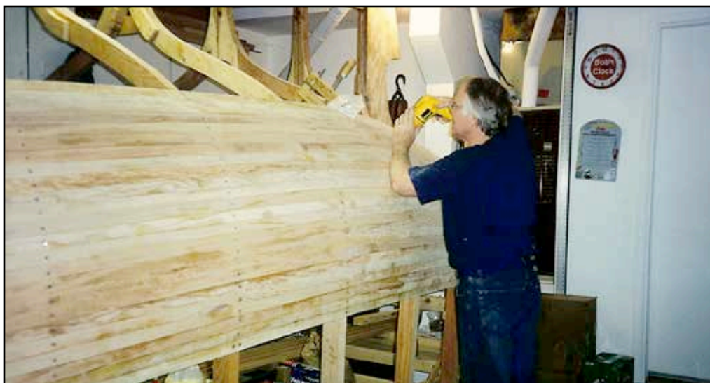
Securing one of the many planks after steaming. Photo: Bob Collier © 2013
