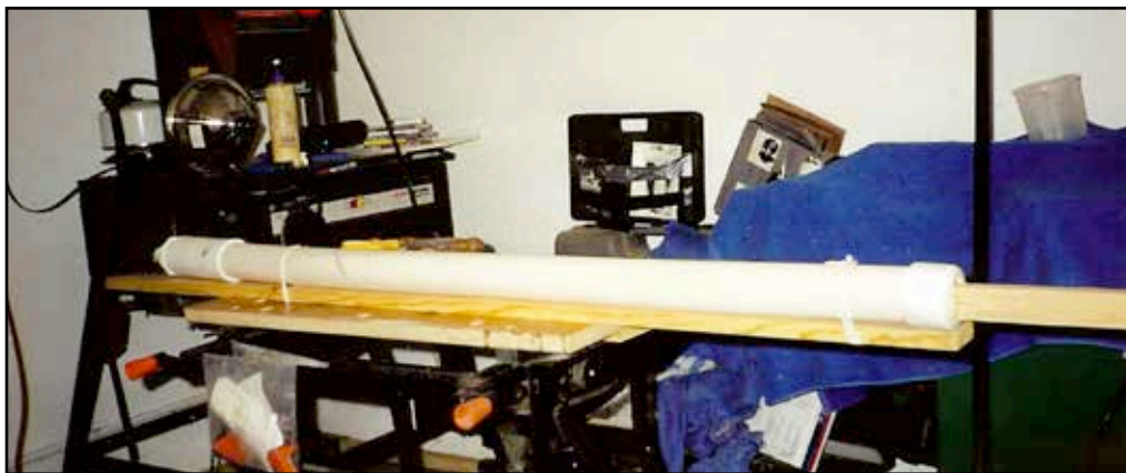
Steaming for an hour was enough to allow bending the plank into shape. Photo: Bob Collier © 2013
