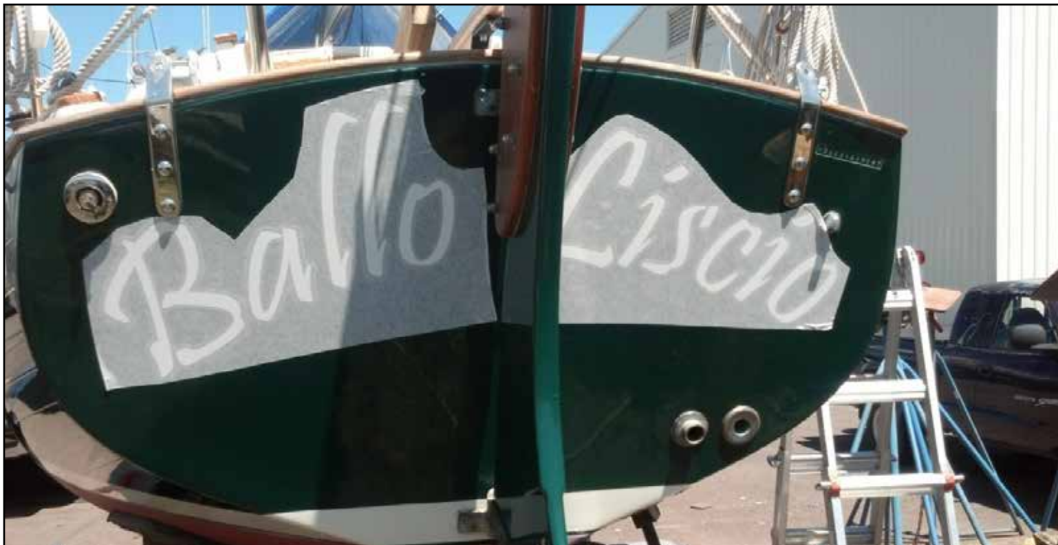
Step One: Determine layout location. Step Two Apply soap to hull and squeegee air out from under letters. Photo: Daryl Clark © 2013
