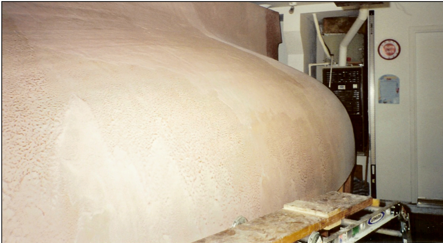
A layer of epoxy and glass powder followed the fiberglass. Photo: Bob Collier © 2013
