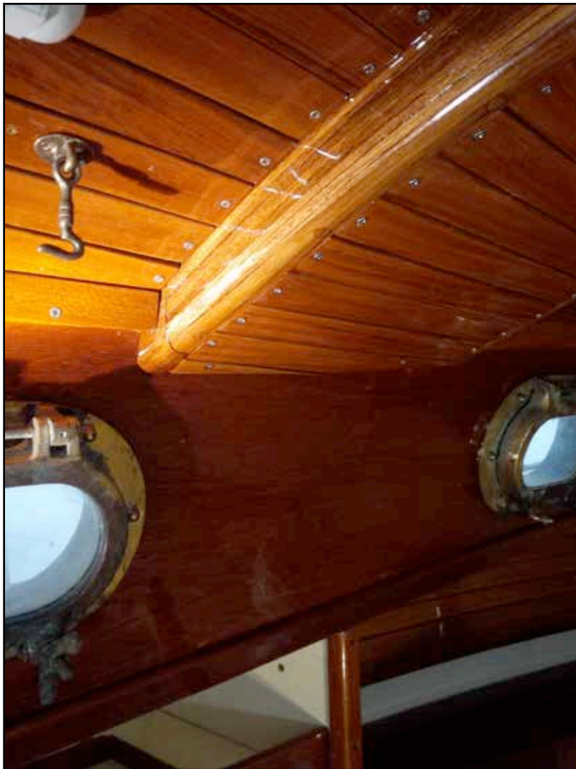
The vinyl headliner was replaced with teak. Photo: Ian Williams © 2013
