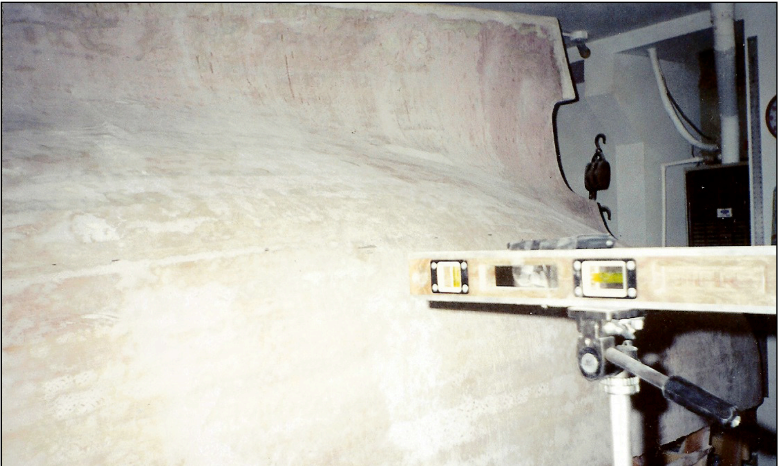
The waterline was marked using a tripod, level, and laser pen. Photo: Bob Collier © 2013
