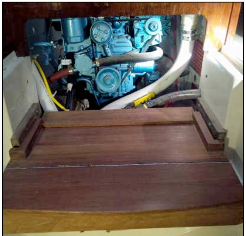
The new Nanni diesel engine and a custom step. Photo: Ian Williams © 2013
