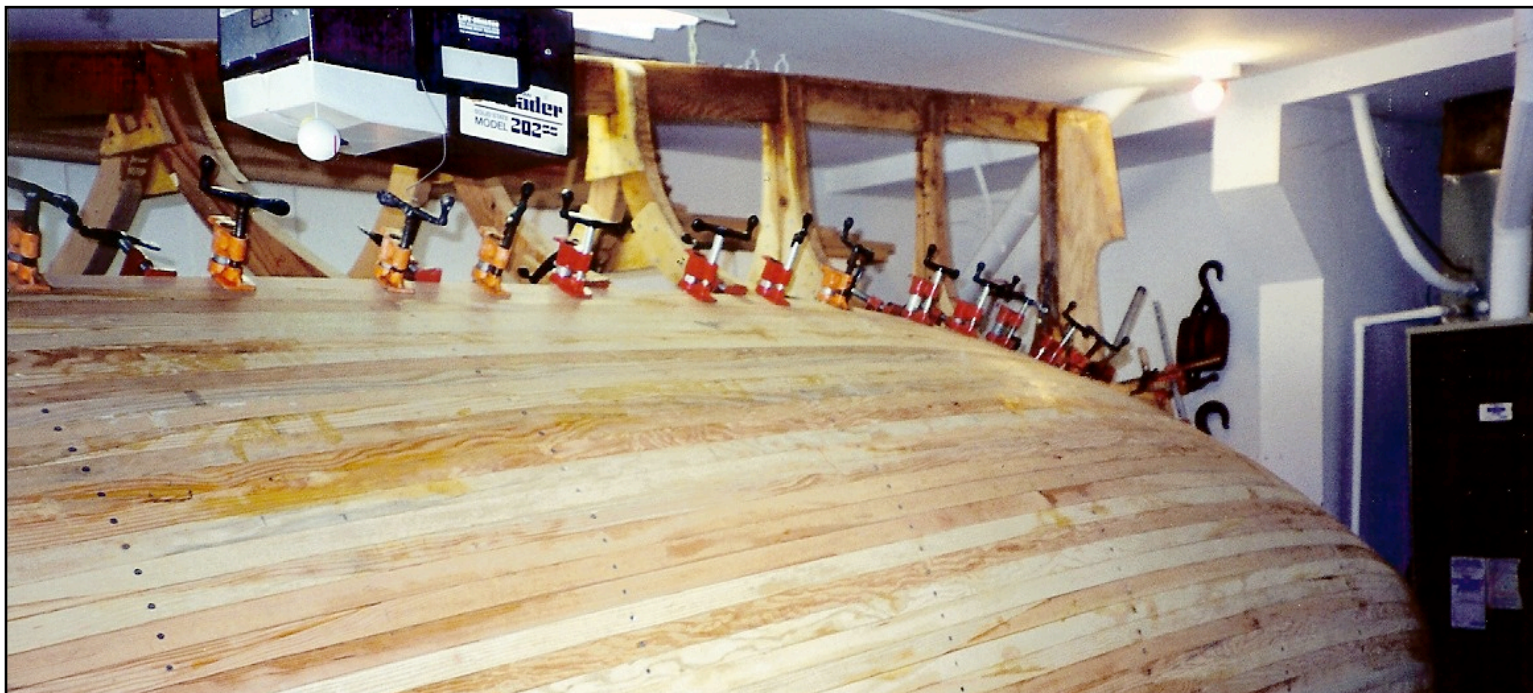
Quite a few clamps were required to hold each plank as it was added to the hull.
