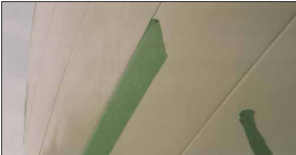
Finding and marking the many nicks, scratches, and gouges for filling and fairing. Photo: Ian Williams © 2013
