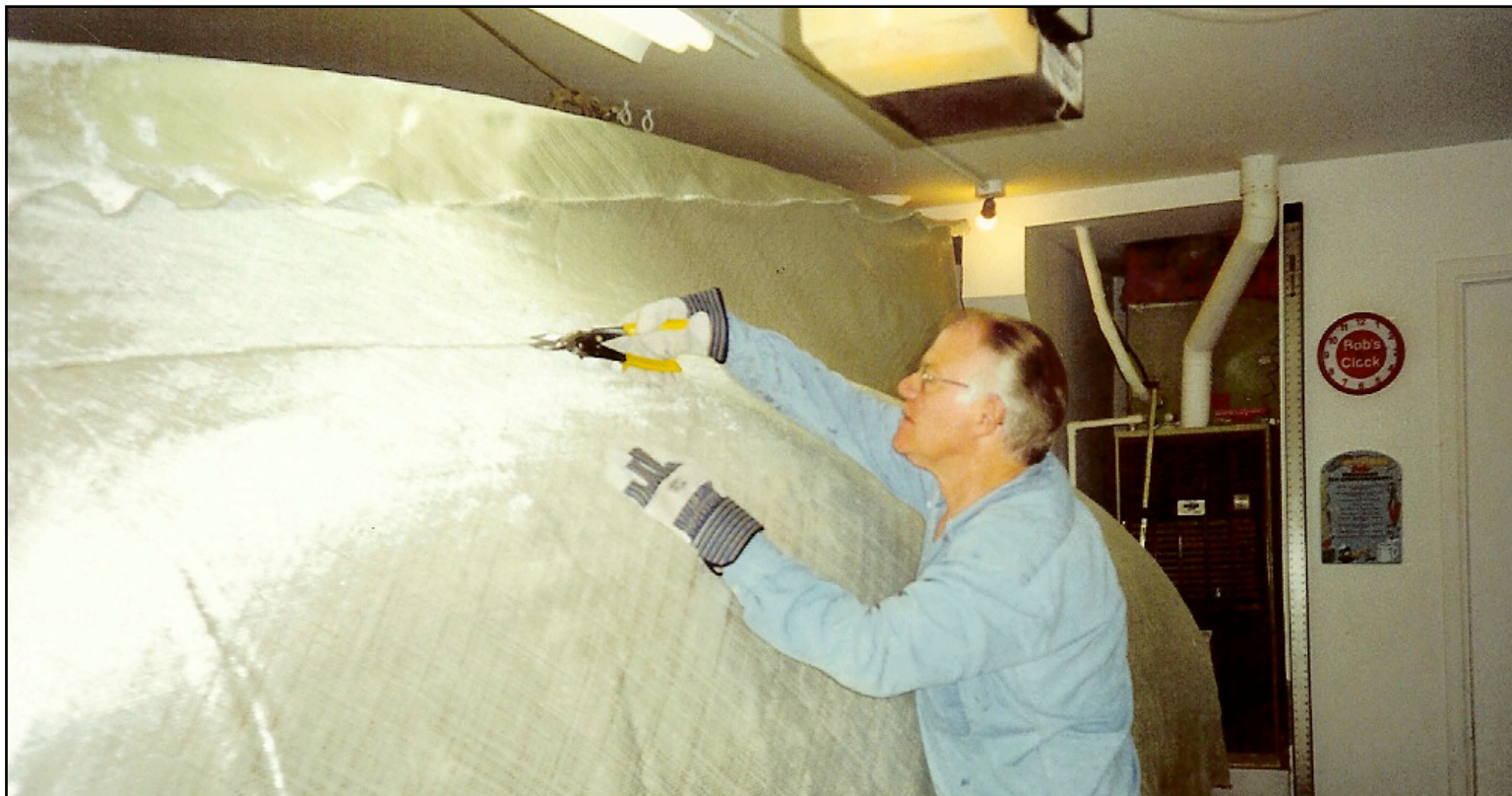
Cutting the fiberglass to shape. Various types, weights, and number of layers of fiberglass was used.
