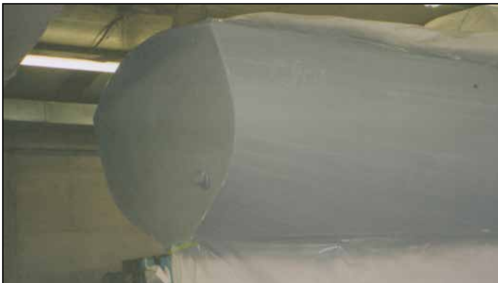
The first step was applying a gray primer coat to the topsides. Photo: Ian Williams © 2013
