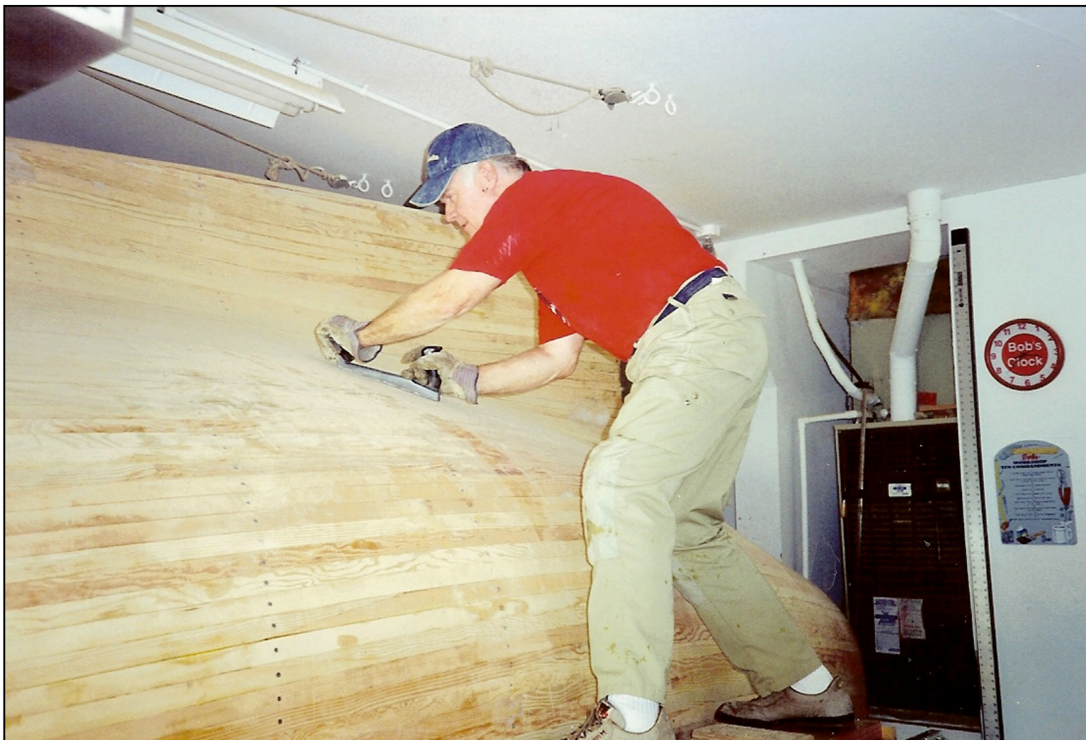
Sanding was next, ranging from the surfum to finer grades of sandpaper using circular and belt sanders.
