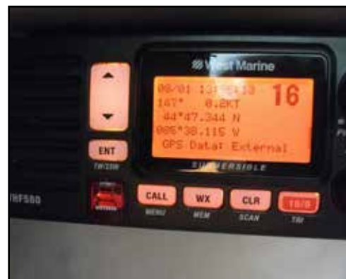
The "puck" G.P.S. antenna provides G.P.S. information to my new marine radio. Photo: Randy Richardson © 2013
