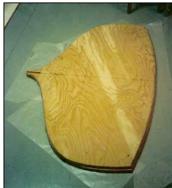
Two layers of 3/4" plywood make up the transom.
