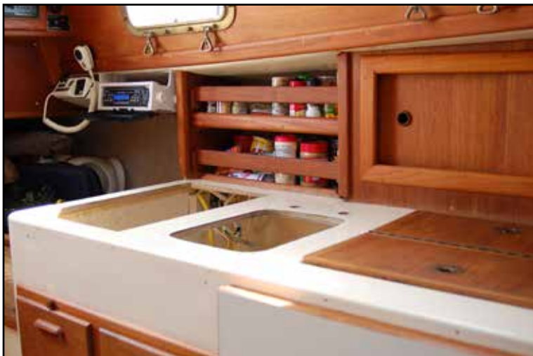
The stove, sink, and facets were removed first. Photo: Jerry Ragland © 2013
