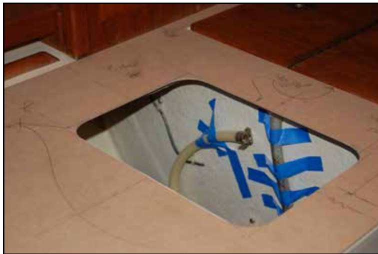
A template was used to determine the measurements. Photo: Jerry Ragland © 2013
