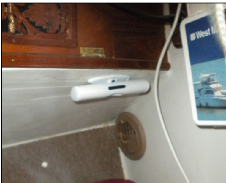
A cabin vent was installed as well. Photo: Bill Cartwright © 2013
