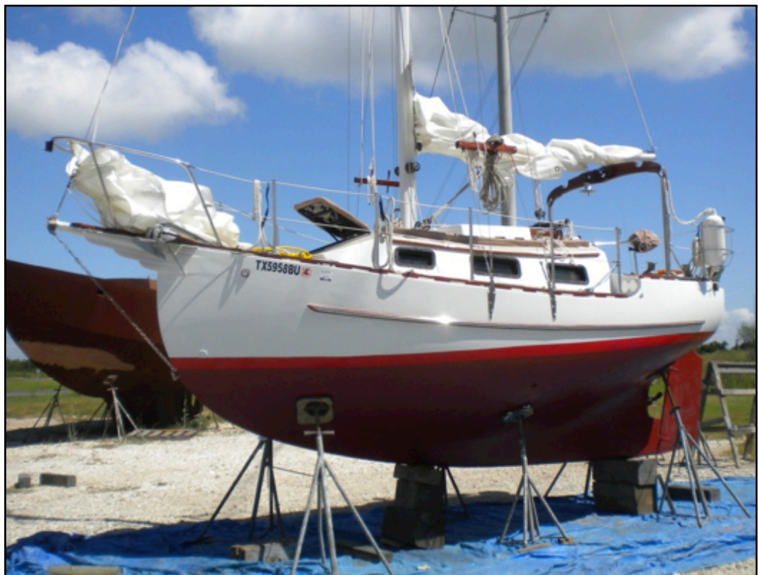
After the maiden voyage, the waterline was adjusted to match the actual balance. Photo: Bill Cartwright © 2013
