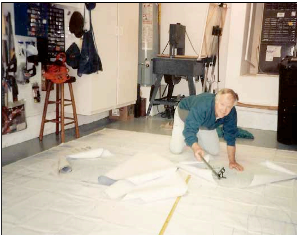
Working on the lofting for my Flicka. Photo: Bob Collier © 2013
