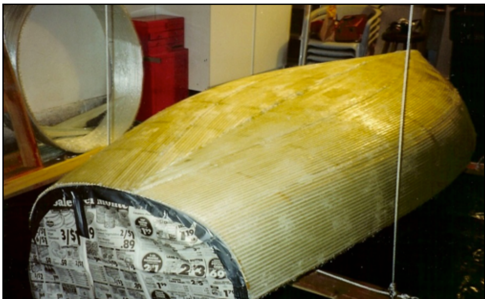
Working with C-Flex to build a small day sailor. Photo: Bob Collier © 2013
