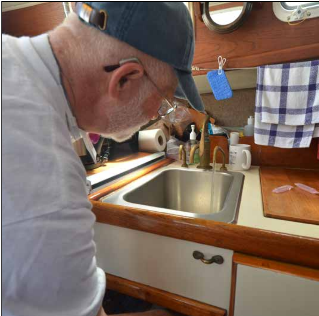
The hose from the small pump is plumbed to another spigot in the sink. Photo: Tom Davison © 2013
