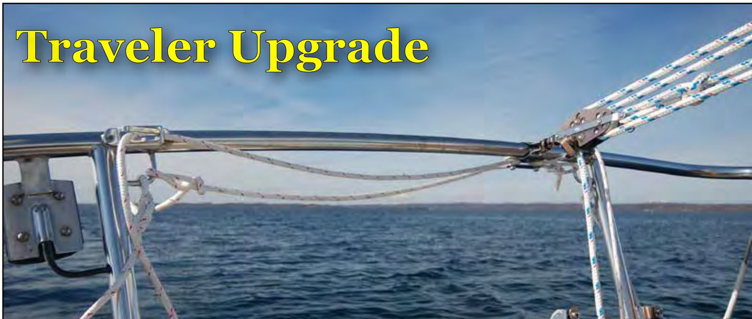
The stock mainsheet traveler of the Flicka on s/y ZANZIBAR . Photo: Tom Davison © 2013
