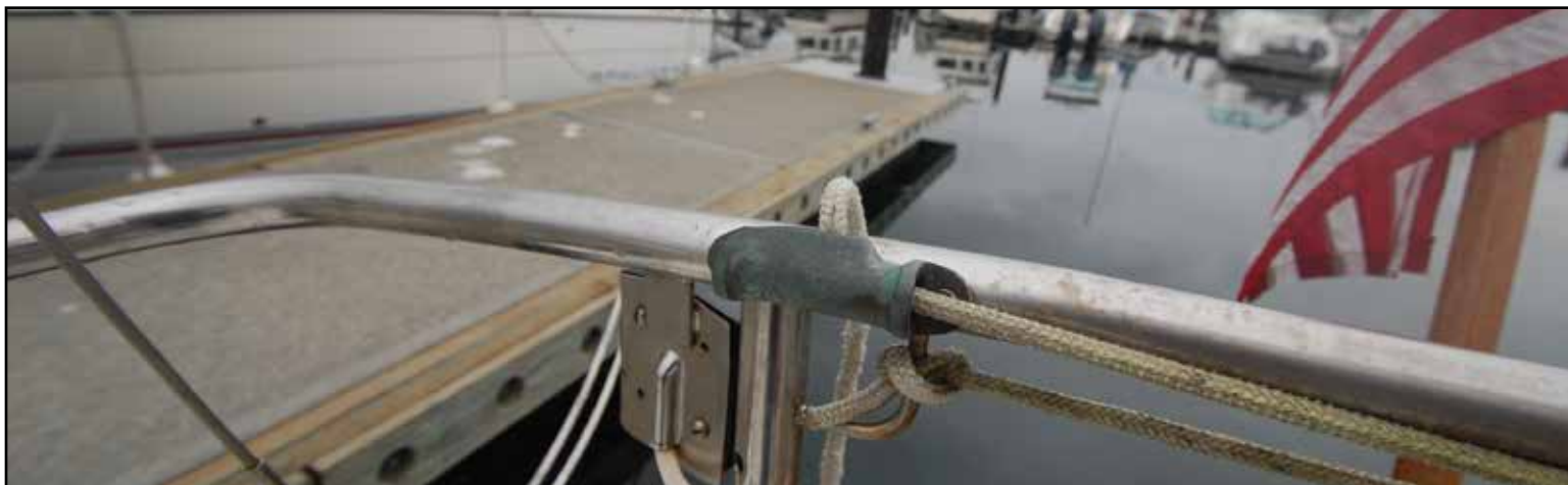
The bronze tubular jam cleats aboard s/y BLUE SKIES . Photo: Tom Davison © 2013
