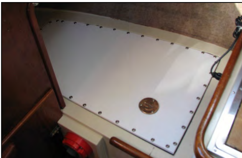
The new water tank cover is a great upgrade over the plywood. Photo: Dick Behan © 2013
