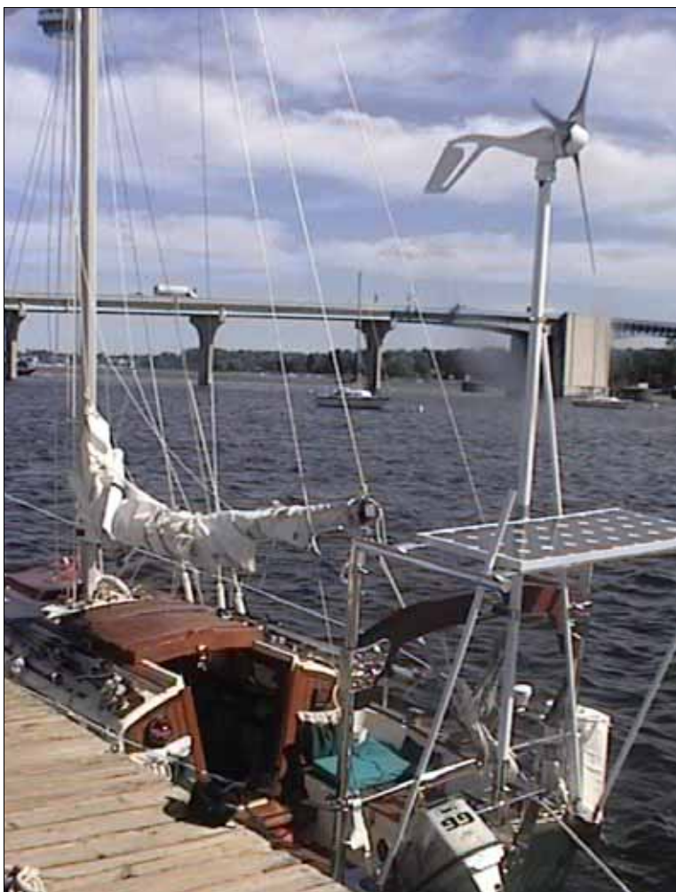
The gallows supports a wind generator and solar panel.
