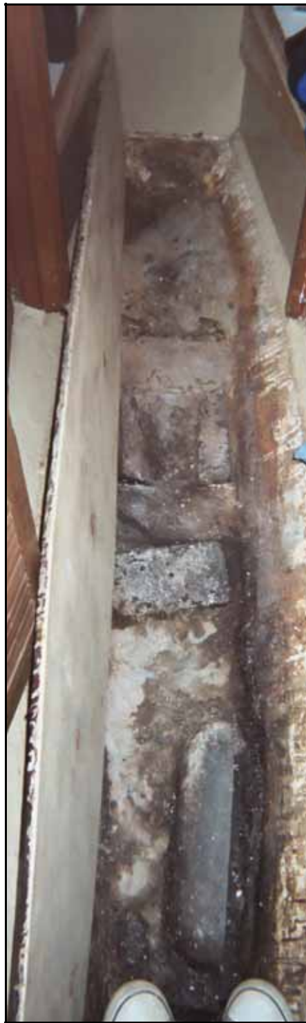
Lifting the floorboard showed some of the ballast.
