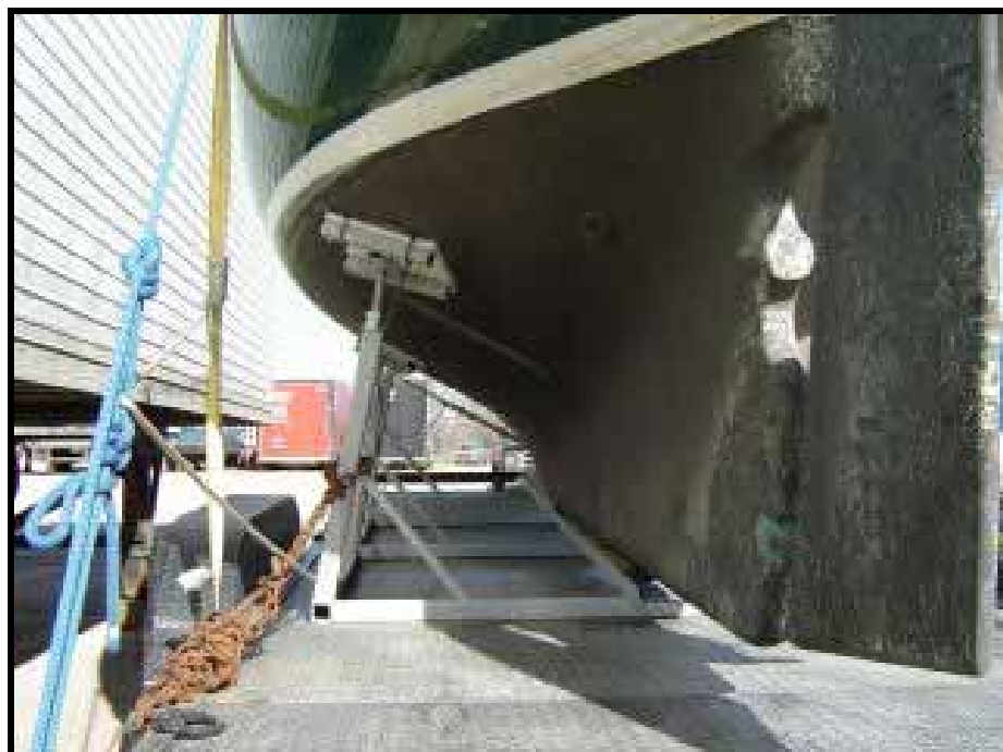
Chains are used to secure the cradle in place, ropes and straps secure the Flicka to the cradle and trailer.
