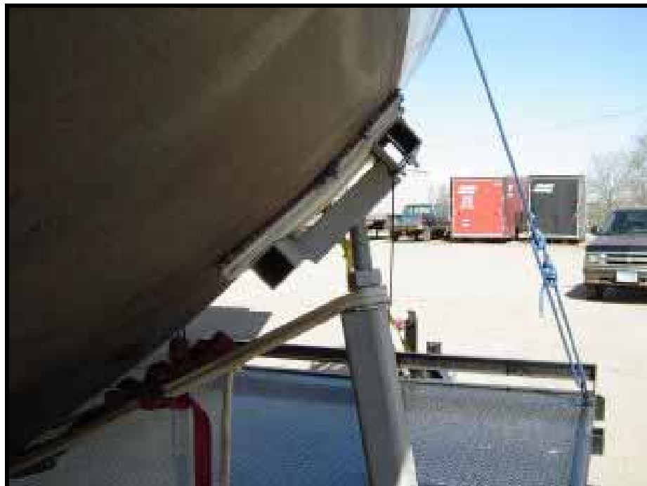
The trailer pads allow the plywood to flex and adapt to the shape of the Flicka's hull.
