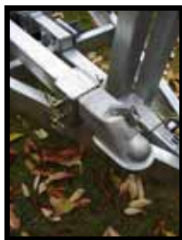
The trailer extension is secured at the tongue of the trailer.
