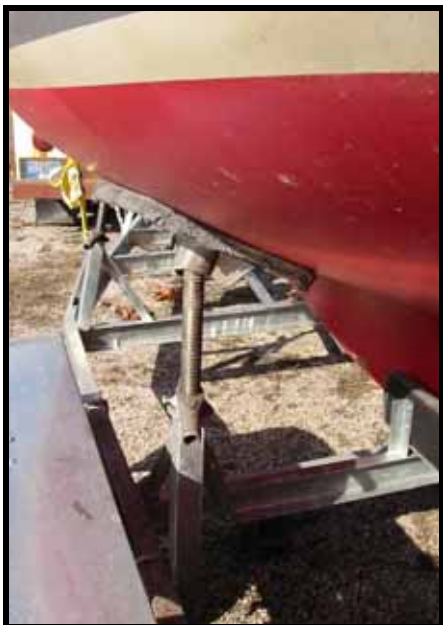
The center pad is probably the most important one in terms of placement of the Flicka on the trailer.
