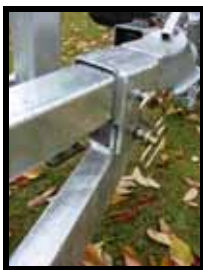
The trailer extension is secured at the tongue of the trailer.
