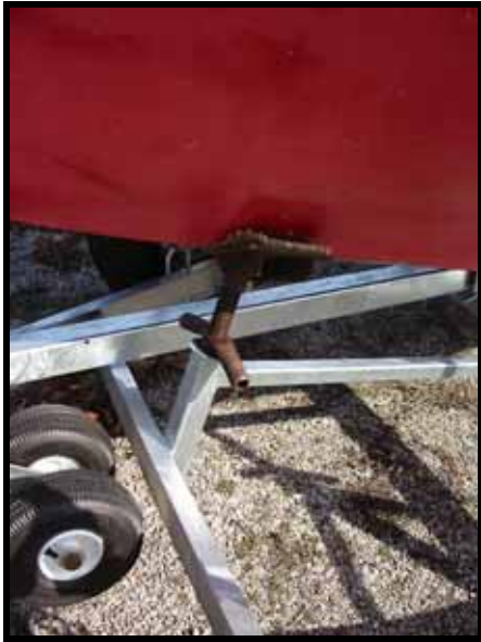
The forward-center flat pad was replaced with a v-shaped pad. This should help loading the Flicka next summer.
