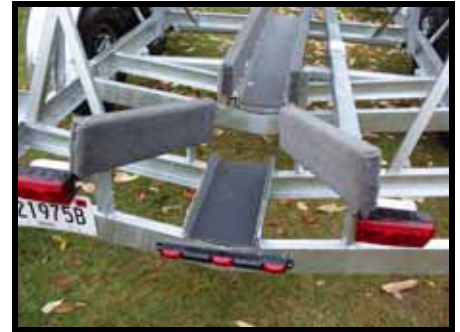
Standard D.O.T. lighting, keel guide and keel supporting.
