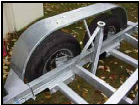
Torsion bar axles and amidships hull support.
