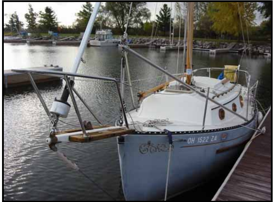
Tom Grimes' Flicka BEN MAIN, Jr. uses a couple of aluminum poles and the mainsheet to lower the mast to the deck.
