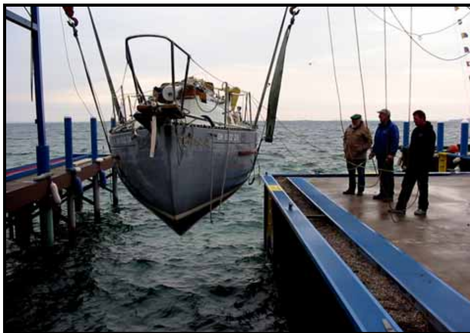
BEN MAIN, Jr. required several attempts to get on the trailer. In the end, we discovered that the support pads were not close to the placement required to properly support the Flicka.
