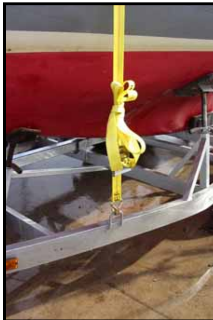
Two straps were used to secure the Flicka to the trailer.
