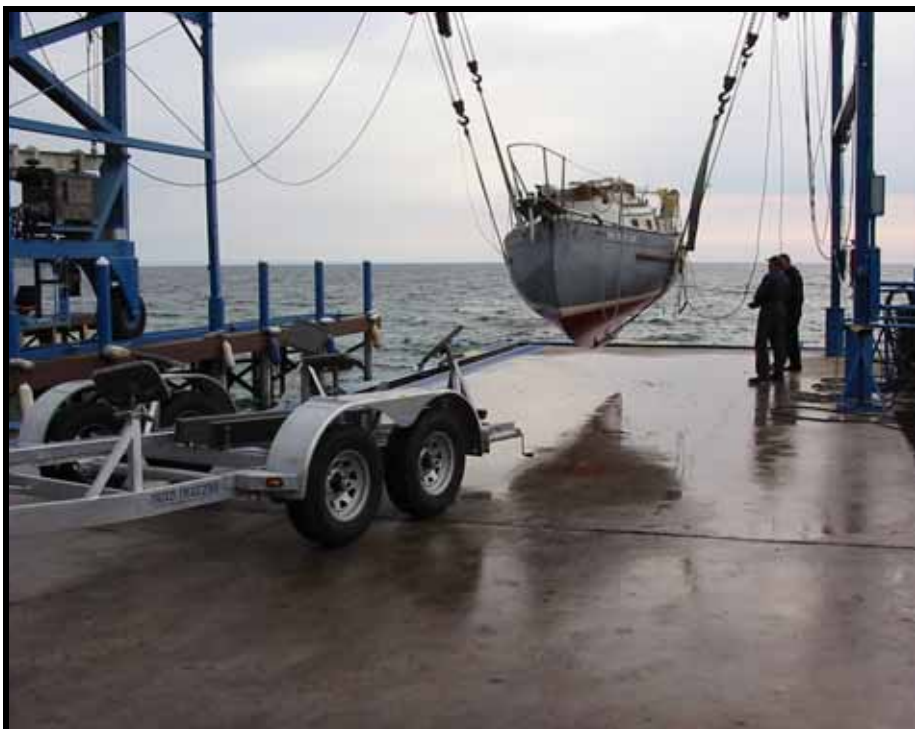
A California built Flicka meets a Connecticut built trailer for the first time. Note the height of the support pads on the trailer. Photo: © Tom Davison 2003
