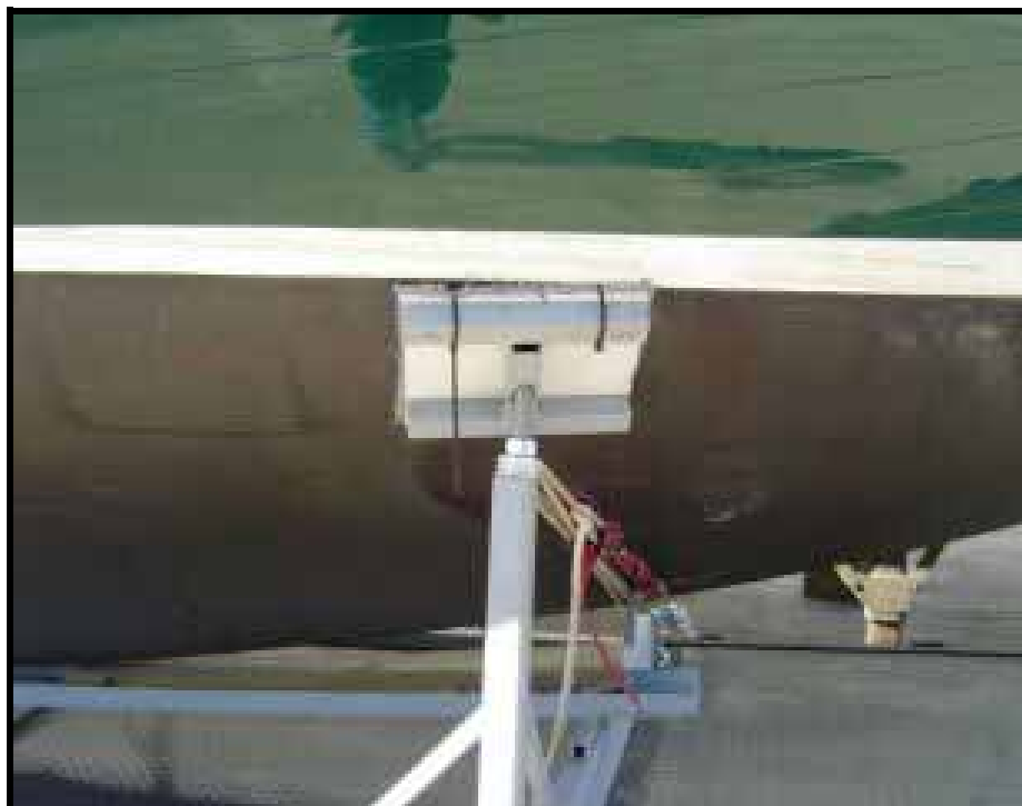
Another support will be added to the cradle at the forward crossbeam to support s/y HAPPY LITTLE GIRLS 2 .
