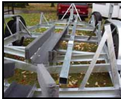
Carpeted keel support and keel guides.
