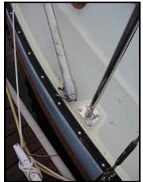
The lower end of the poles are connected to the slotted rail of the Flicka with a couple of small links.
