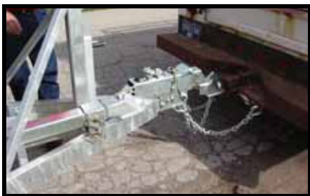
The coupler is a 10,000 pound model to fit a 2 5/16 inch ball.
