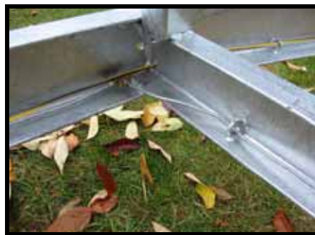
Secured brake lines & wiring.
