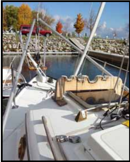
ABOVE & MIDDLE —Two small wood supports hold the mast, boom, gaff, and stays'l boom.
