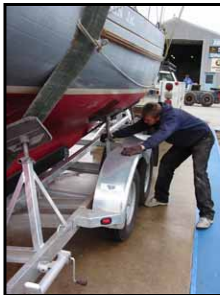
After lowering BEN MAIN, Jr. onto the trailer, each of the pads were adjusted.
