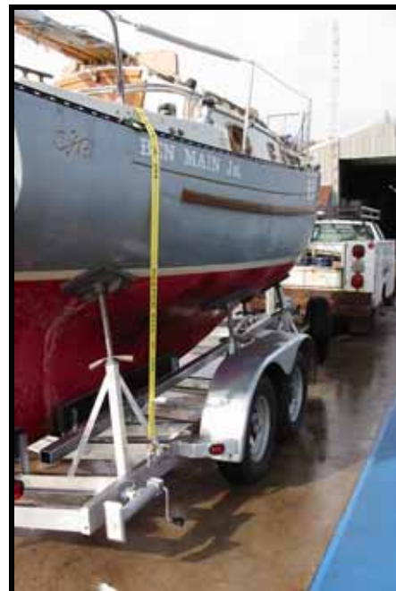
Two straps were used to secure the Flicka to the trailer.
