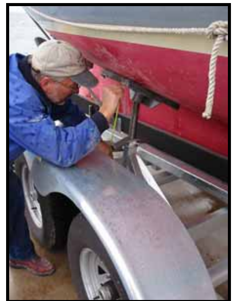
The pad height was measured and adjusted as required to center the hull on the trailer.
