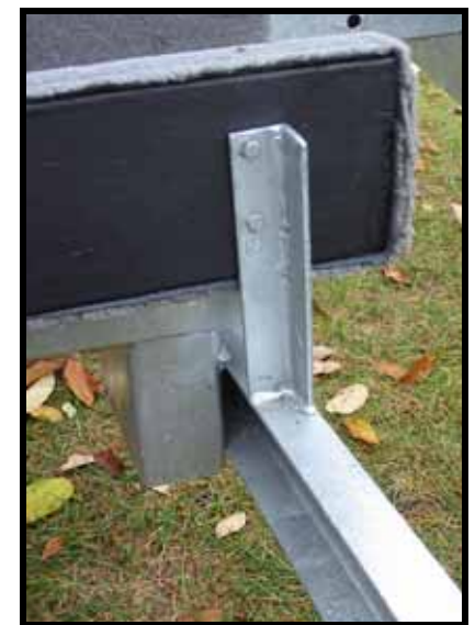
The keel guide and base of the keel support.
