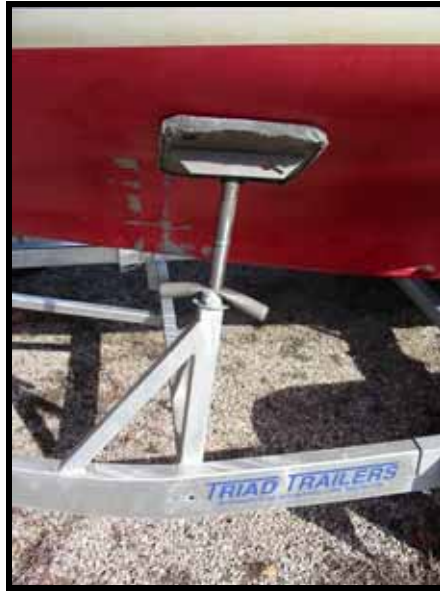
This is the port-forward pad, referred to as pad # 1 on the Triad trailer.
