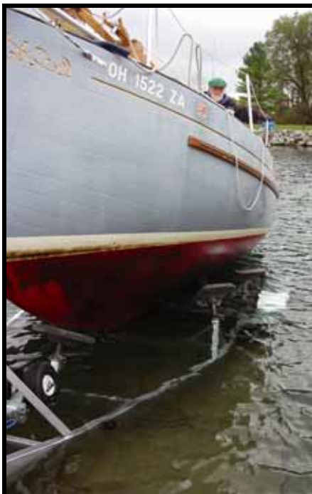
BELOW —The bottom line was that the pads were a little short of the required height to support the Flicka.
