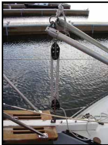
The main sheet was used to lower the mast to the deck. This works perfectly allowing you easily control the weight of the mast and rigging.
