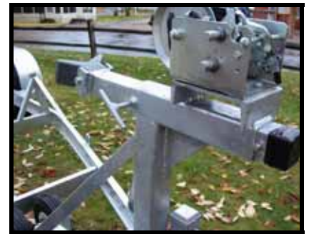
The adjustable bow stop allows you to balance the load.
