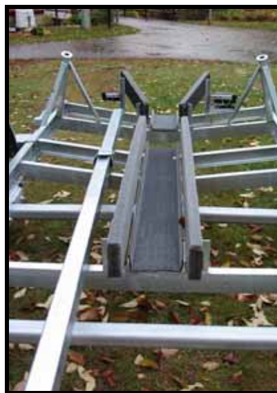
The tongue extension lies to the side of the keel support.
