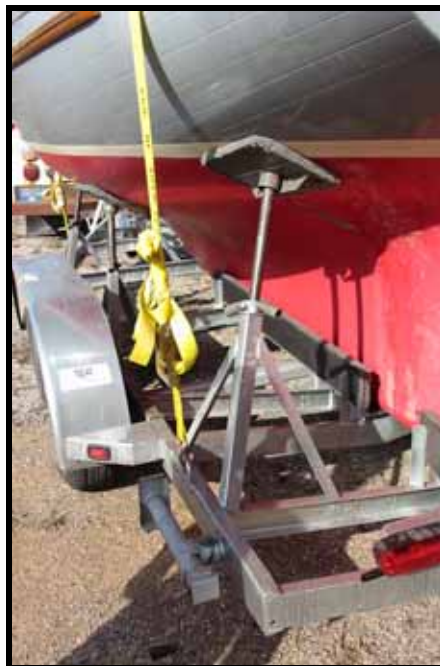
The aft-port flat pad was extended to meet the hull. Also, note the gap in the guides that allows placement of the lift strap.
