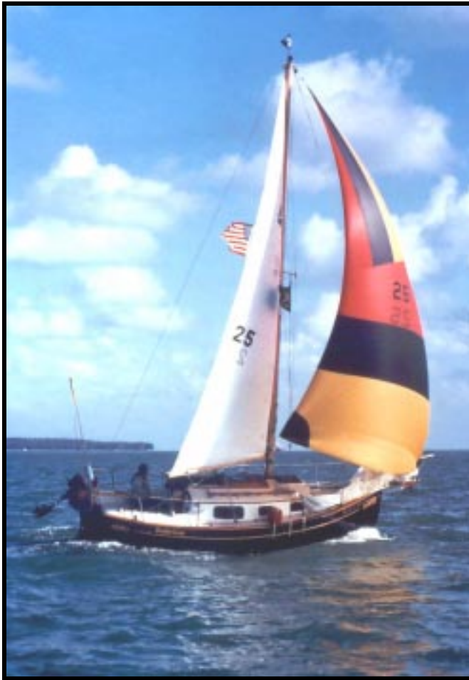
SABRINA reaches at full steam with her colorful 150% reacher/drifter. © Bruce P. Bingham 1978 & 2003.
