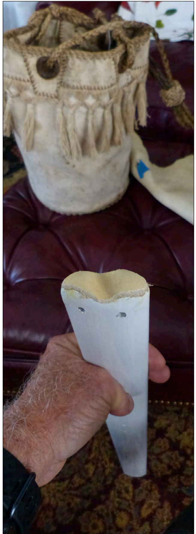
After filing a nock in the epoxy filler end cap, I glued on a piece of goatskin to prevent chafe on the new synthetic standing rigging. Photo: Jamie White © 2020
