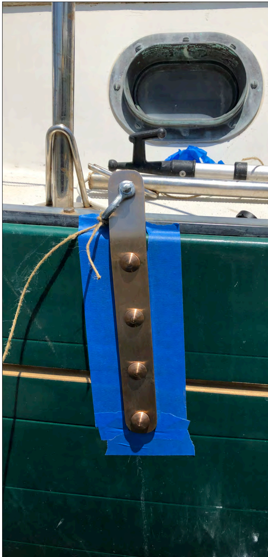
Portside chainplate installed and bedded with 3M 4000 polyurethane sealant. Photo: Jamie White © 2020
