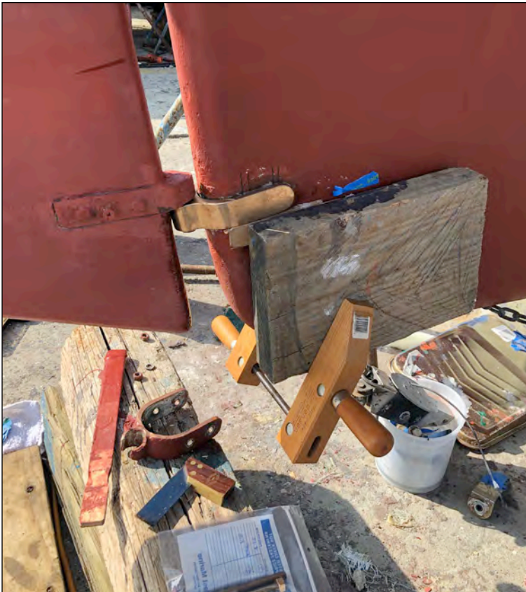
A wooden block was used as a stop for fitting the gudgeon. Photo: Jamie White © 2020
