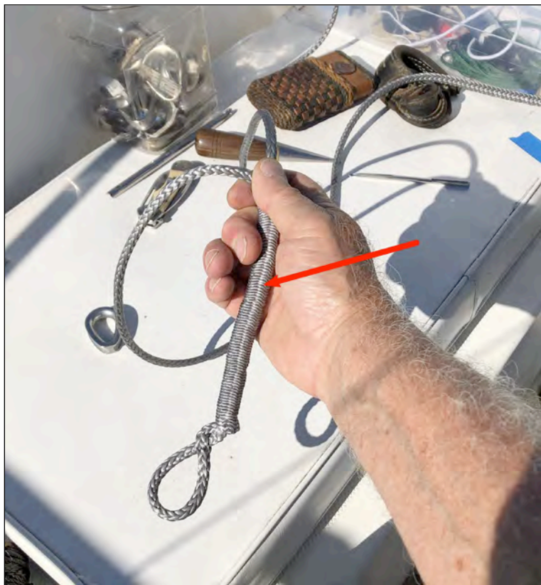
Step N - Slide the standing part cover down the tail until there is about 9" or about 1/3 of the tail exposed depending on line diameter. This 9" section will be tapered before being drawn back into the standing part braid. This taper will ensure that the splice tapers nicely into the standing part. A lump at the termination of the splice will cause a weakness in the finished splice.
