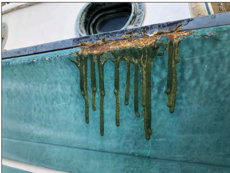
Previous repair along the starboard deck / hull joint. Photo: Jamie White © 2020
