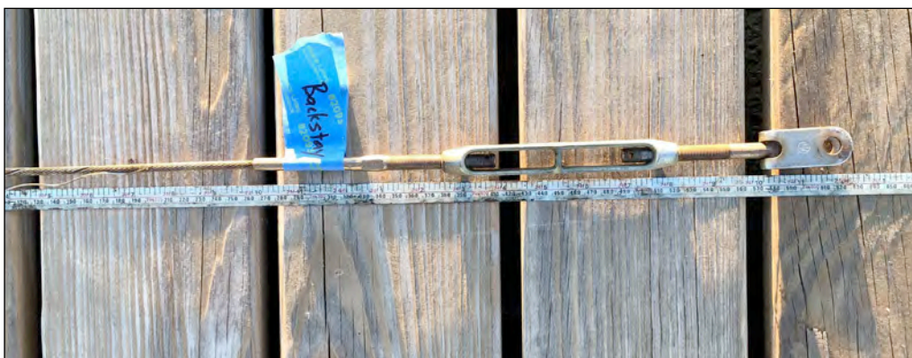
When measuring rigging, I ensure the turnbuckles are set at between 1/3 to 1/2 of their take-up. Photo: Jamie White © 2020
