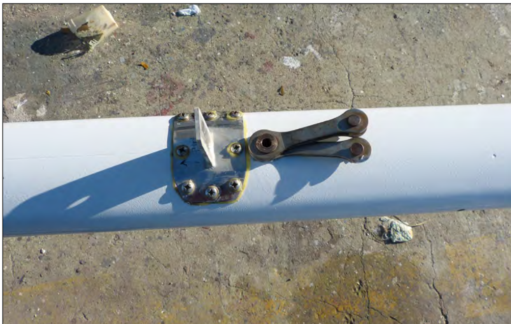
After removing all the old paint, I sanded the aluminum mast using 220 grit paper followed by a mild acid etch of white vinegar and water. Then I applied an aluminum etching primer followed by three topcoats of white INTERLUX–Brightside® One-Part Polyurethane Paint. After it dried, I affixed the hardware, bedded with LanoCote® to combat galvanic corrosion where dissimilar metals are fastened together.
