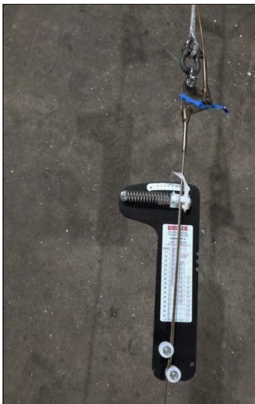
The pre-tension the splices for DULCINEA's rigging was to almost 10% of minimum breaking strength to reset the braid.
