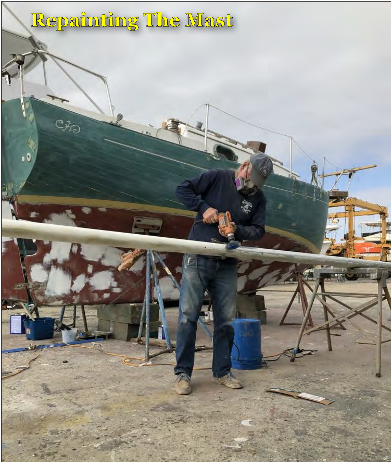
Paint removal from the mast during the refit of Pacific Seacraft Flicka # 302. Photo: Ruth Downes © 2020
