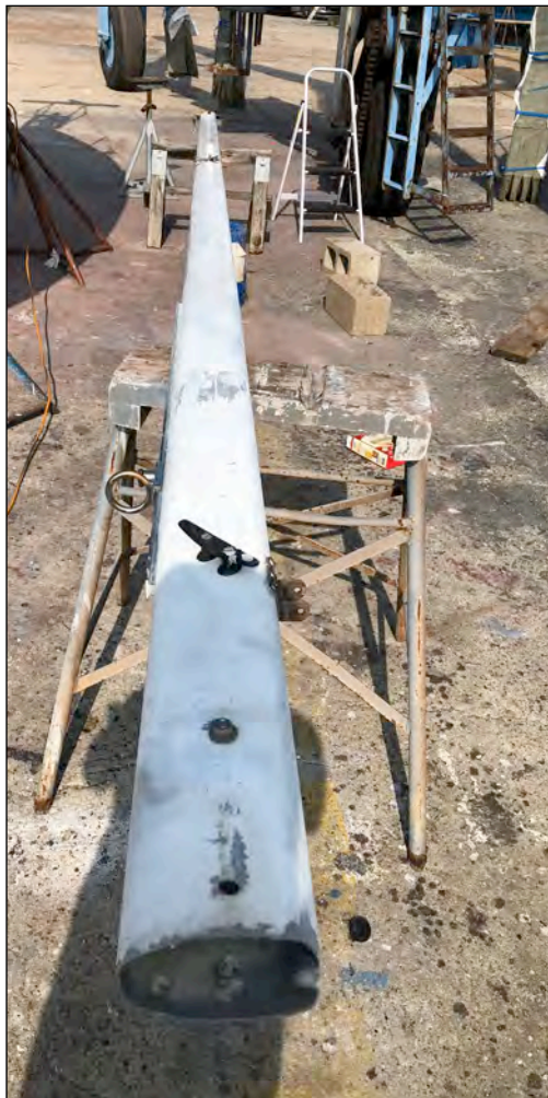
A mast looking for a paintbrush. Getting ready to remove all hardware, tracks, and masthead sheave box before removing oxidized coating. Photo: Jamie White © 2020
