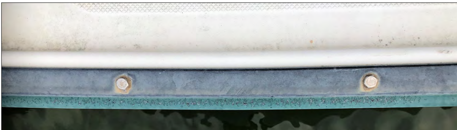
Examples of pinholes in gelcoat at turn of topsides under the toe rail. Photo: Jamie White © 2020
