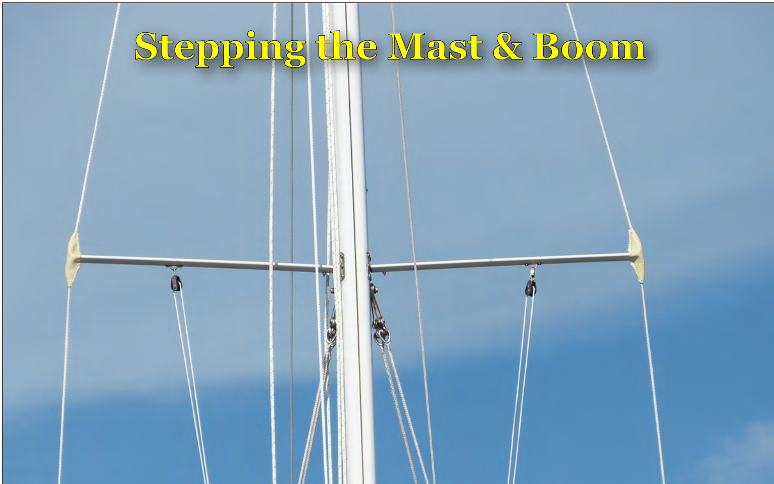
Detail of spreader boots and the new Dyneema rigging aboard s/y DULCINEA .
