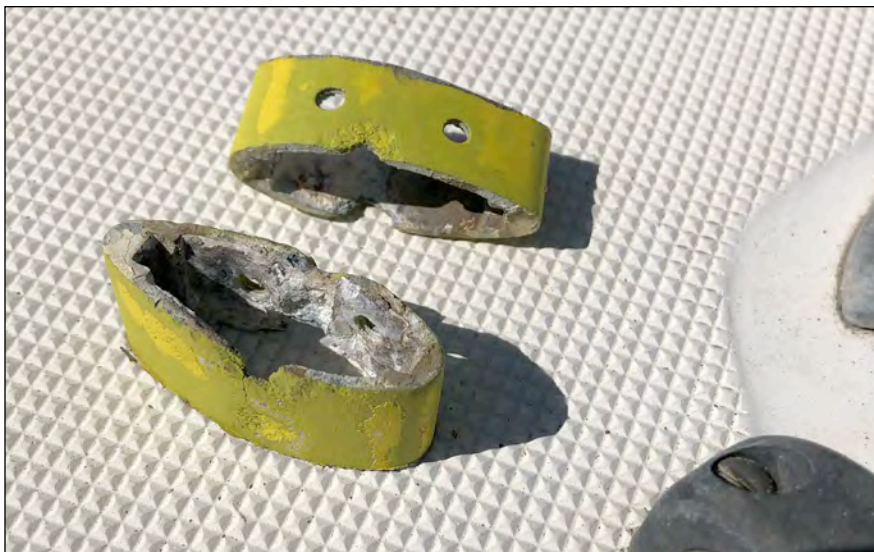
I decided to trim the last 1/2" off the spreaders and built it back up using two-part marine epoxy filler. Photo: Jamie White © 2020
