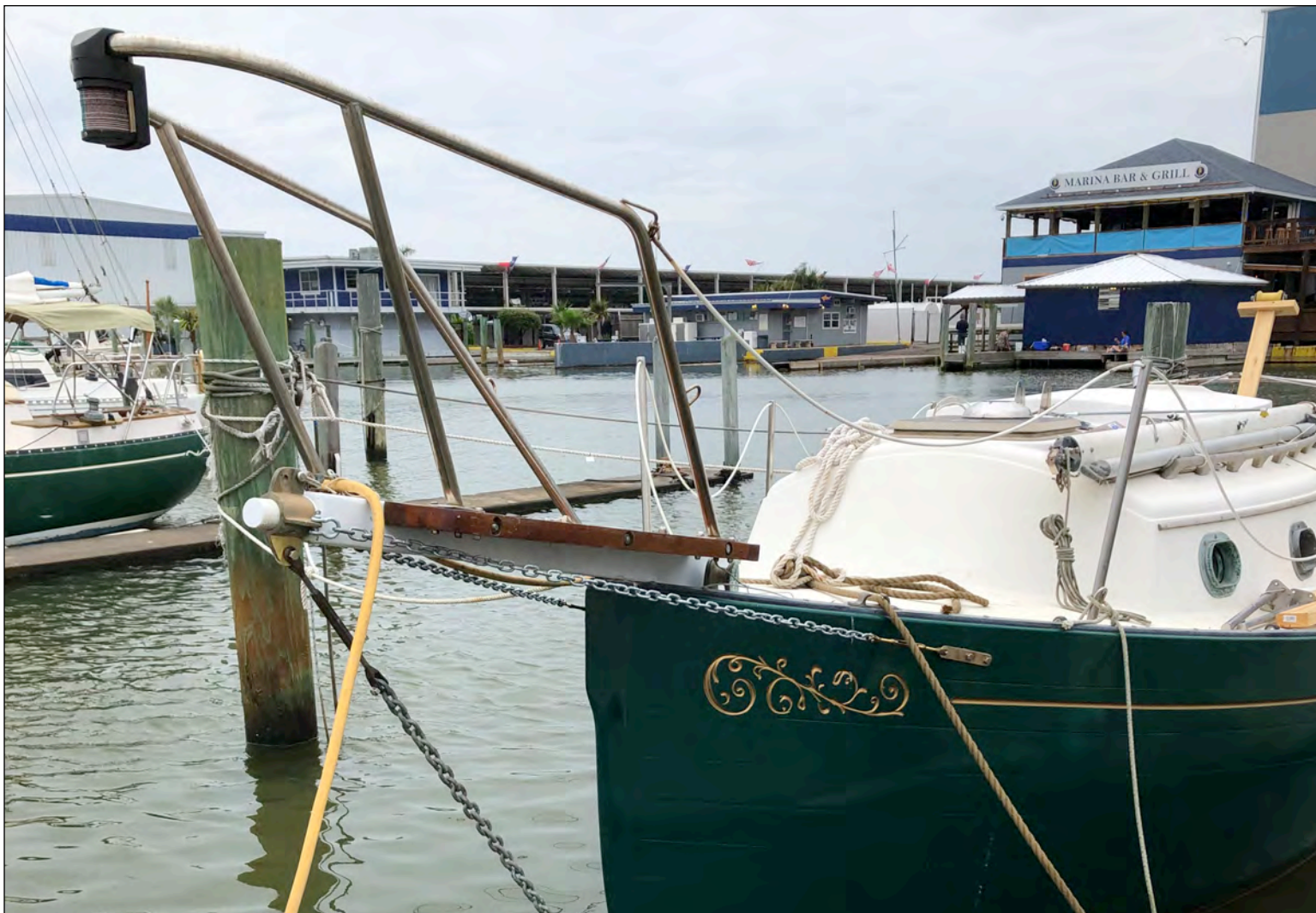
New bowsprit fitted with new galvanized chain bobstay and bowsprit shrouds. Photo: Jamie White © 2020
