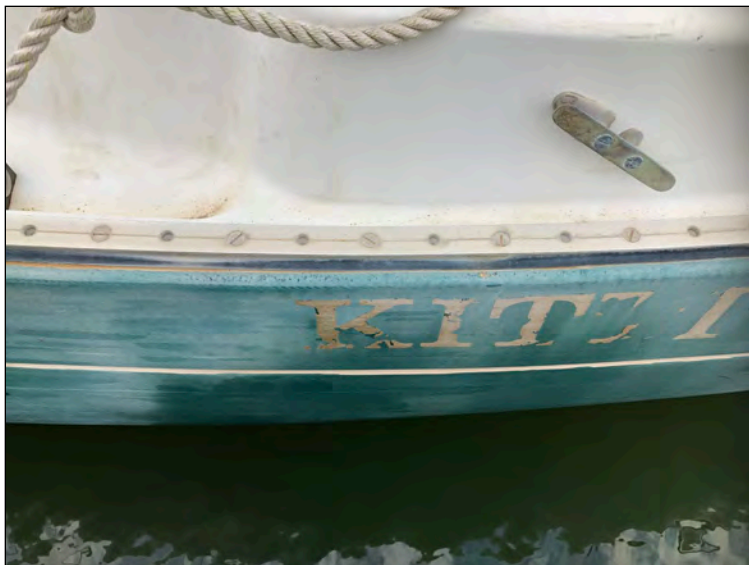
Examples of pinholes in gelcoat at turn of topsides under the toe rail. Photo: Jamie White © 2020
