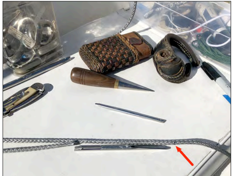
Step G - I determine where to exit the hollow body of the standing part one fid length from the end of the tucking strand. Photo: Jamie White © 2020
