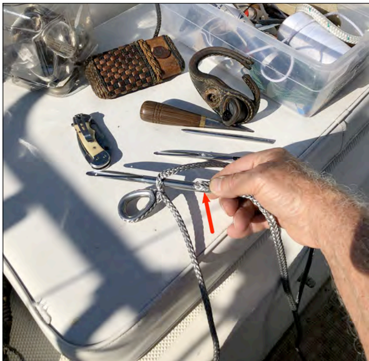
Step B - Second or locking pass. I like to enter about a fid width from the first pass. Note I am passing the already spliced eye (standing part) through the working end leg. To do this, I remove the thimble and squeeze the eye into the Selma fid so the spur on the fid grips the eye.
