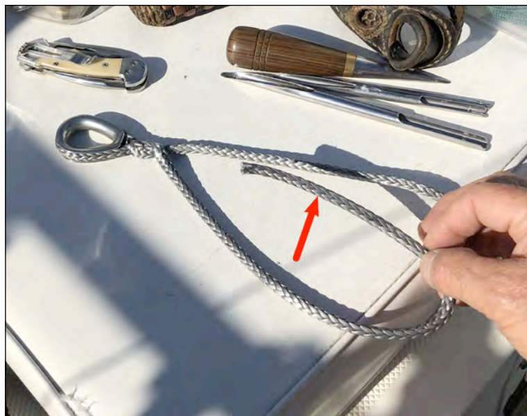
Step E - Complete locking Brummel tucks with the tail ready to be passed through the hollow core of the braid. Some riggers like to taper the tail at this point, but I prefer to taper it after passing it through the hollow body of the standing part
