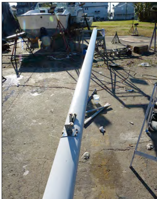
After removing all the old paint, I sanded the aluminum mast using 220 grit paper followed by a mild acid etch of white vinegar and water. Then I applied an aluminum etching primer followed by three topcoats of white INTERLUX–Brightside® One-Part Polyurethane Paint. After it dried, I affixed the hardware, bedded with LanoCote® to combat galvanic corrosion where dissimilar metals are fastened together.
