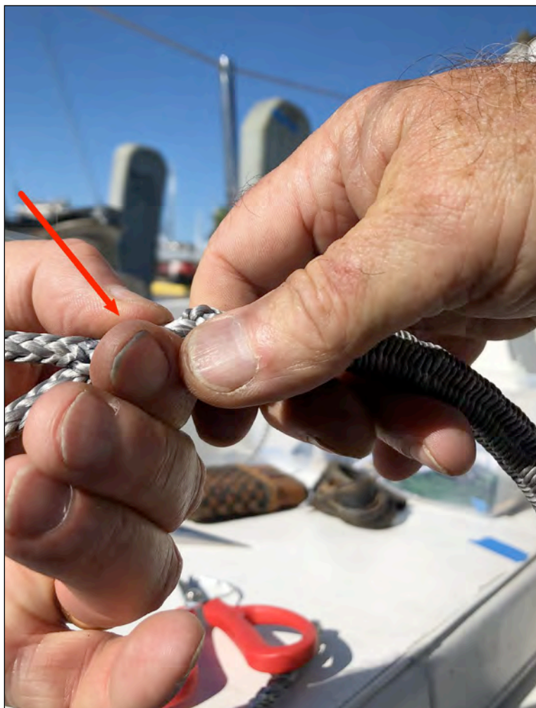
Step R - Hold the splice at the initial Brummel entry and milk the bunched up braid back over the tail. The tail will automatically disappear inside the standing during this operation.
