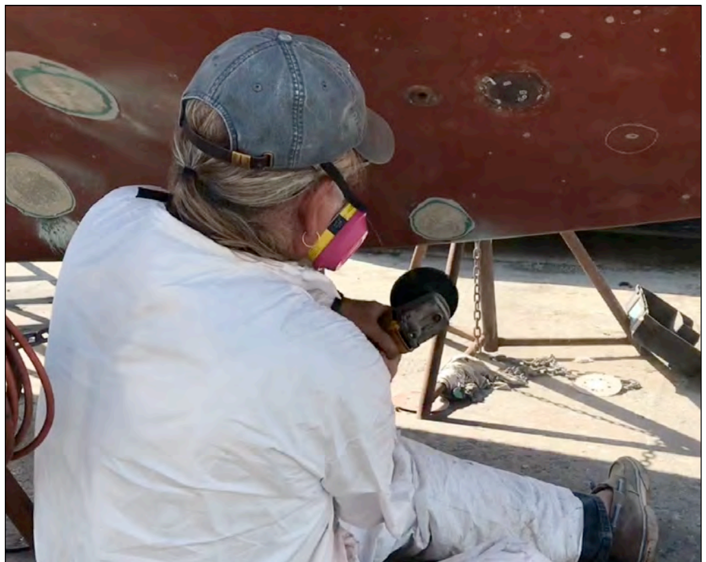
Beginning to grind down a blister until sound fiberglass is found. Photo: Ruth Downes © 2020
