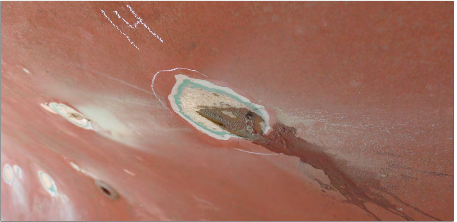
Slowly grinding down until sound dry fiberglass mat or roving is reached. Only several blisters went deep enough to touch the structural roving. Photo: Jamie White © 2020
