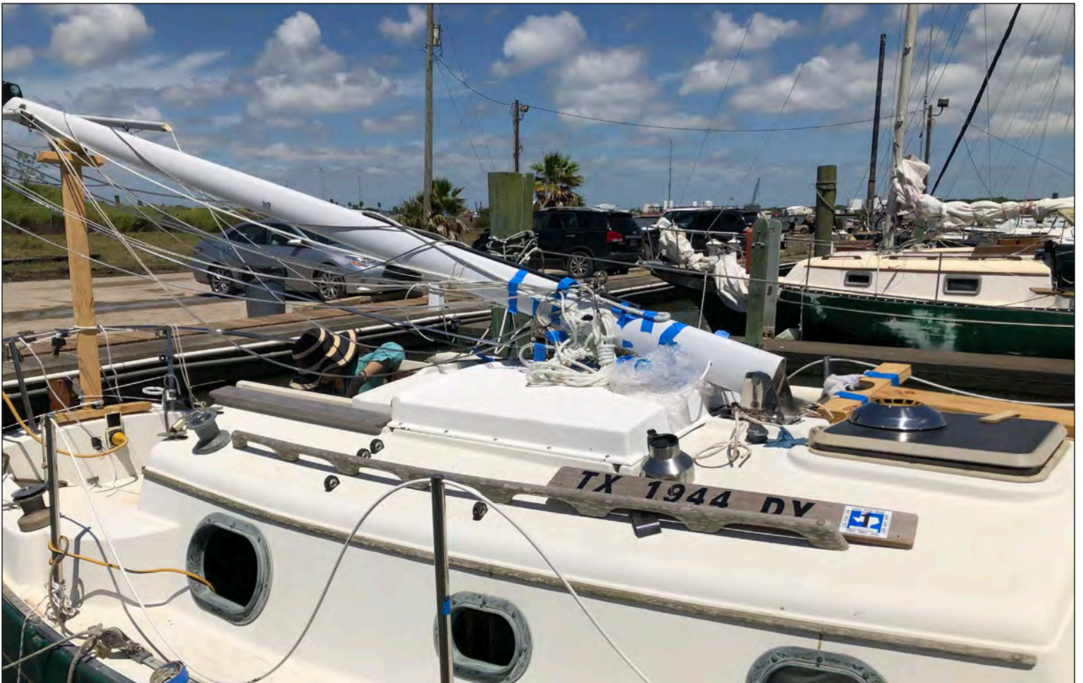
Preparing the mast and rigging for hoisting.
