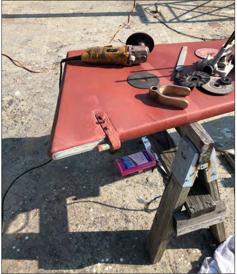
The rudder was lightly trimmed for the new gudgeon. Photo: Jamie White © 2020
