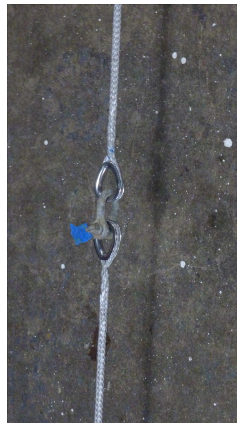
The pre-tension the splices for DULCINEA's rigging was to almost 10% of minimum breaking strength to reset the braid.
