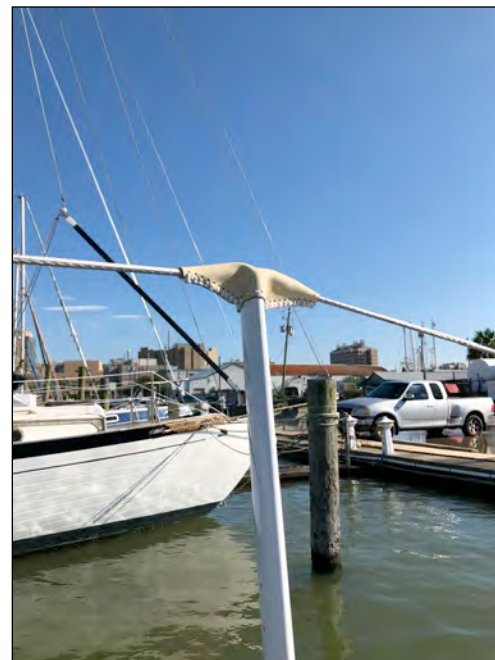
Completed spreader cap boots in place. Photo: Jamie White © 2020
