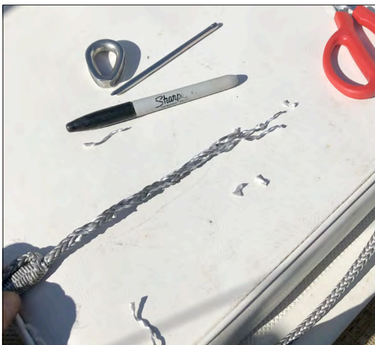
Step Q - Tail tapered and trimmed – ready to be milked back into body of standing part.
