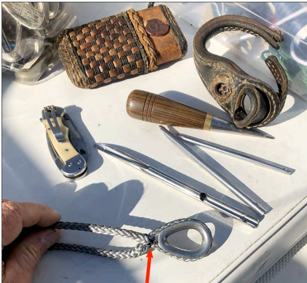
Step A - The first pass of a locking Brummel splice. I like to leave the thimble just slack enough that it can later be removed for splicing the other end or for changing the thimble due to damage while in service.
