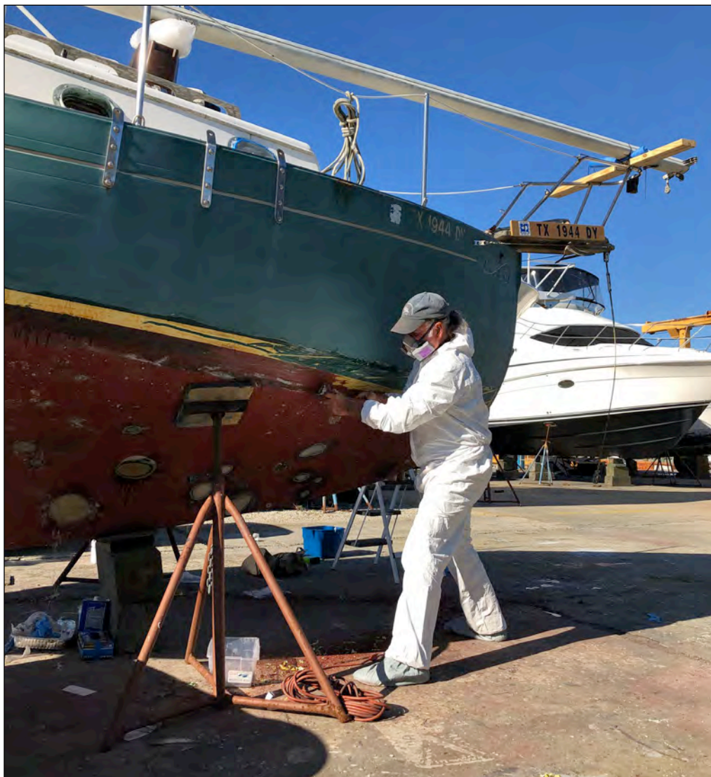
The yellow boot stripe was removed before applying the bottom paint. Photo: Ruth Downes © 2020
