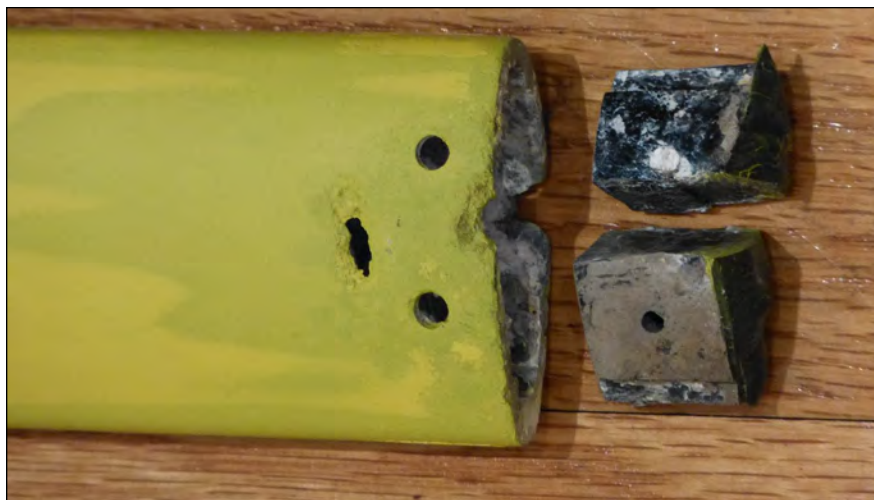
There was corrosion of the aluminum spreader ends Photo: Jamie White © 2020
