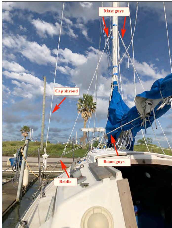
Bruce Bingham's main sheet mid-boom bail modification blends well with using mid-boom stabilizing guys instead of rigging the guys at the end of the boom.
