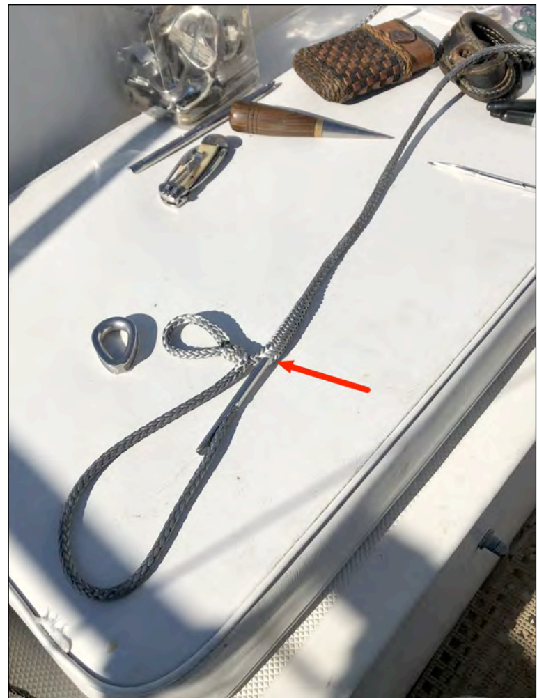
Step I - The fid entering the hollow core of the standing part. Pull just enough tail through to leave a small bight at the thimble. Do not pull the tail tight just yet. Photo: Jamie White © 2020
