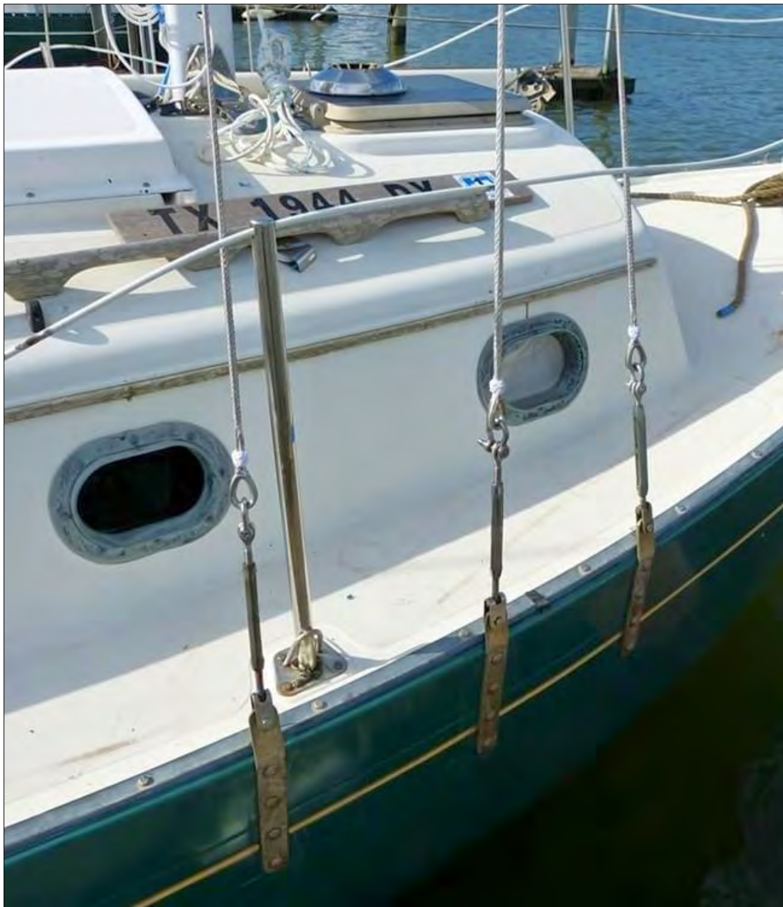
The finished splices with a 4x3 Turks Head as an embellishment. Note – I will mouse all shackles and dog all turnbuckles after the rig settles in after the initial couple of sails. Photo: Jamie White © 2020
