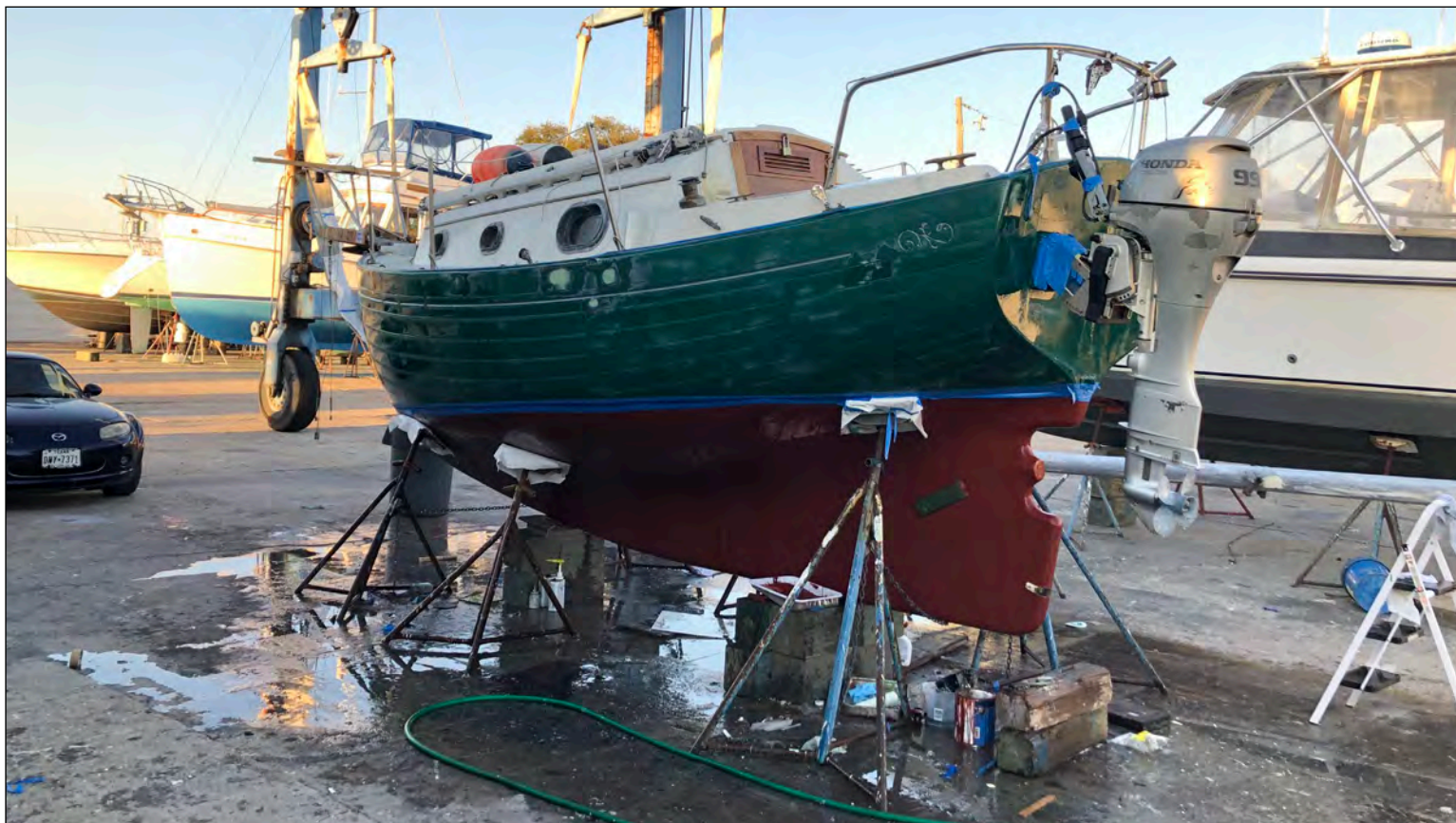
The final coat of bottom paint before priming and painting the topsides. Photo: Jamie White © 2020
