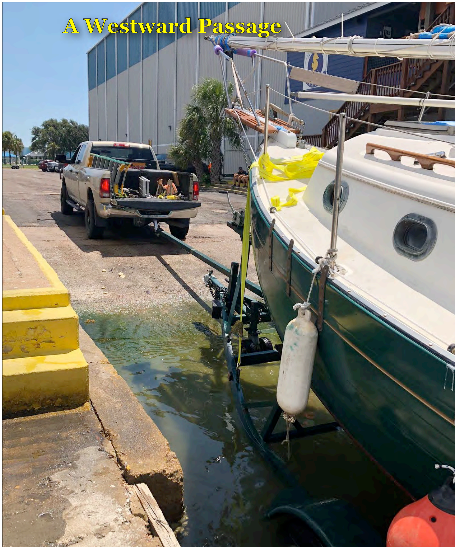
The trailer extension allows the trailer to get under s/y DULCINEA for loading. Photo: Jamie White © 2020
