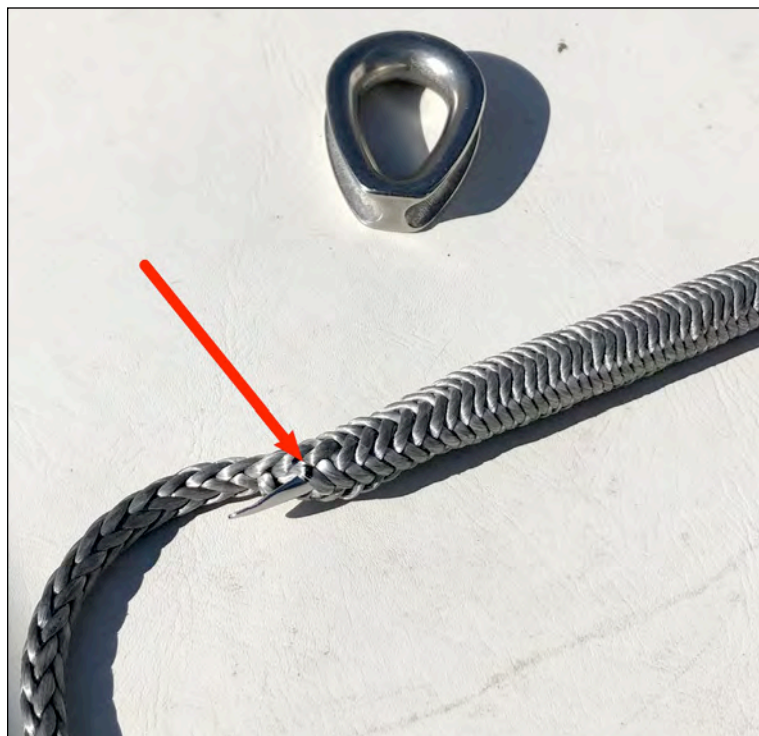
Step J - The fid exiting at the one and a half fid length mark. Photo: Jamie White © 2020
