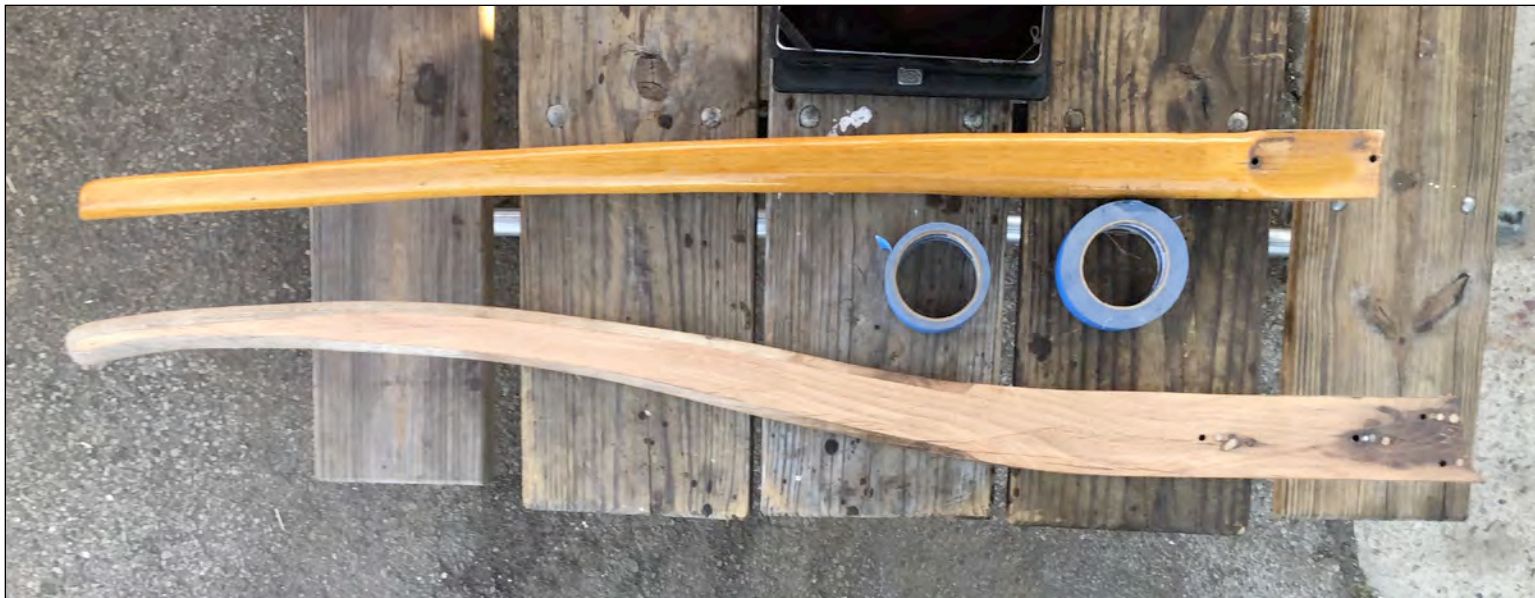
Reshaping the tiller. The tiller at top of photo is a spare tiller I purchased at Minney's that will serve as a back up or emergency tiller. Photo: Jamie White © 2020
