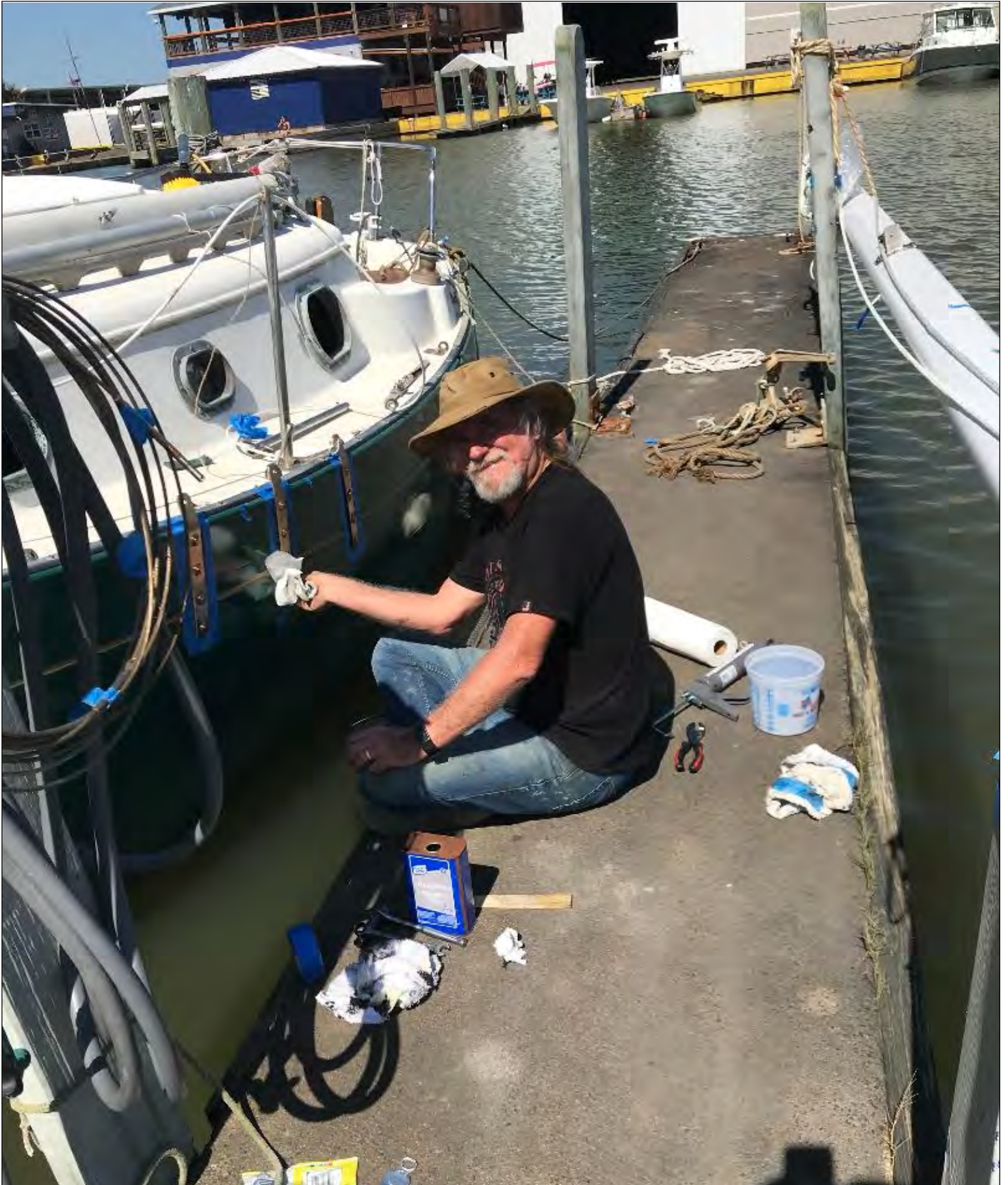
Replacing the chainplates at the dock. Photo: Ruth Downes © 2020
