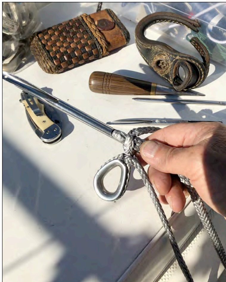
Step C - Note I am passing the already spliced eye (standing part) through the working end leg. To do this, I remove the thimble and squeeze the eye into the Selma fid so the spur on the fid grips the eye.
