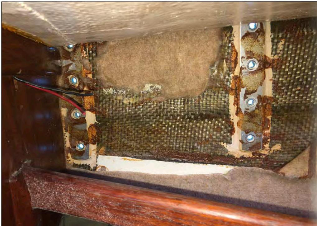
The hull liner carpet was partially removed when I took over stewardship of DULCINEA so it was simple to remove the rest of it to gain access to remove and then tighten the carriage bolts. Photo: Jamie White © 2020
