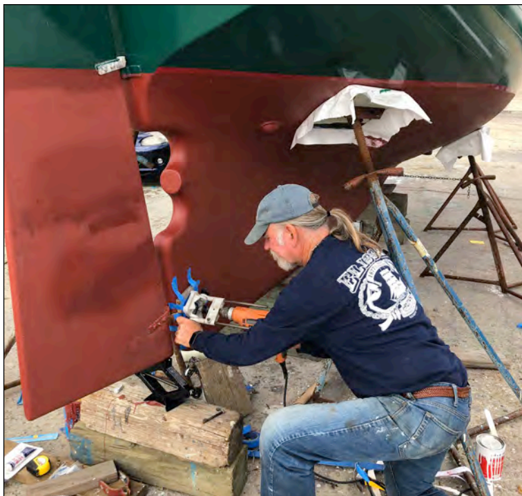
A long shank drill bit was required. Photo: Jamie White © 2020
