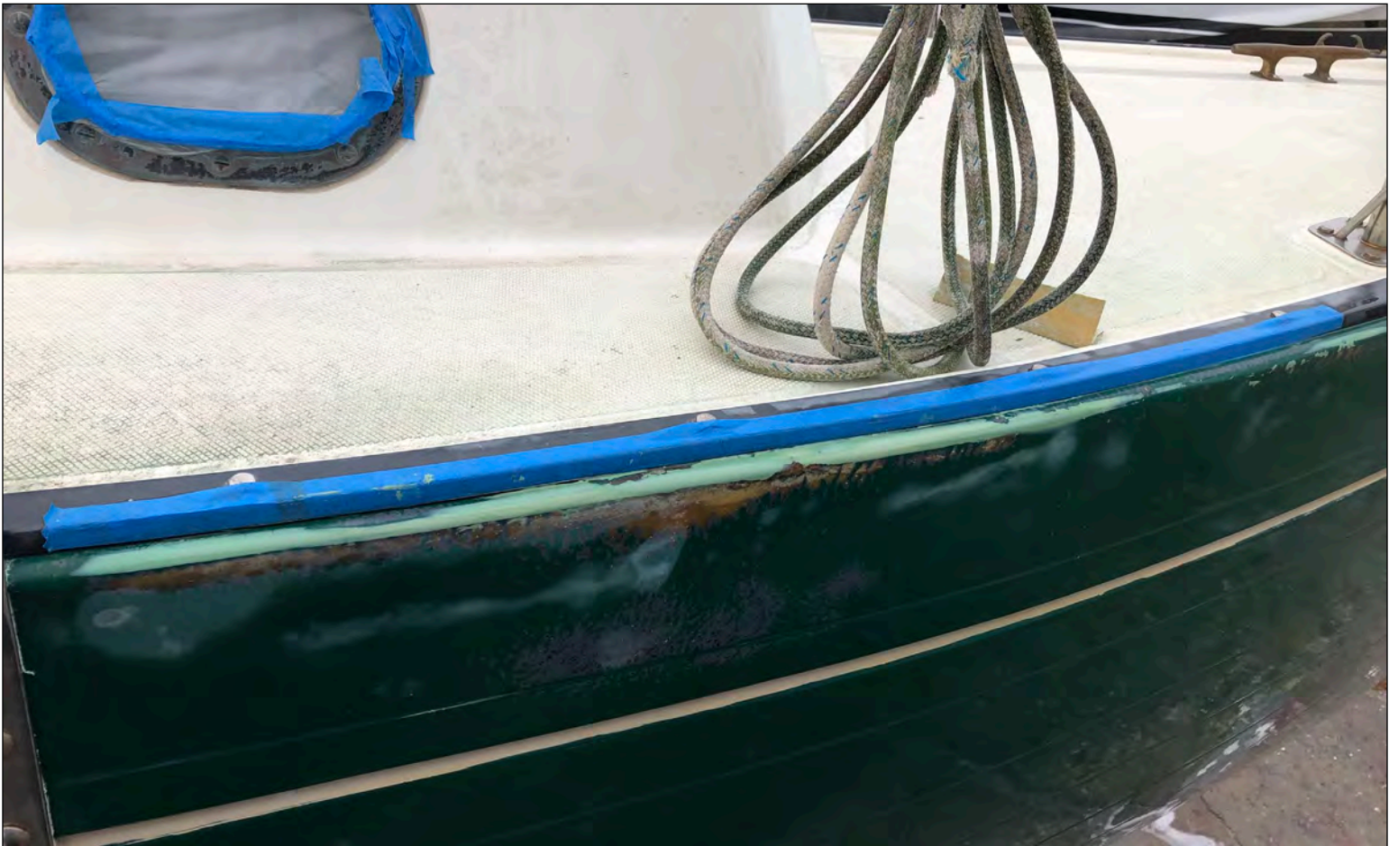
Repairs to the gelcoat on the starboard hull at the deck connection. Photo: Jamie White © 2020
