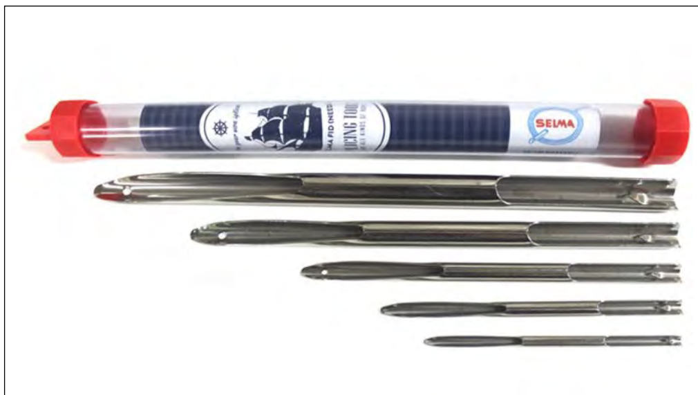
The Selma splicing fids set used on the Dyneema rigging of s/y DULCINEA . Photo: Jamie White © 2020
