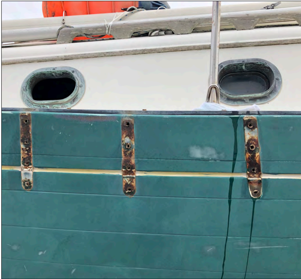
Port view of the hull after removal of the chainplates. Photo: Jamie White © 2020
