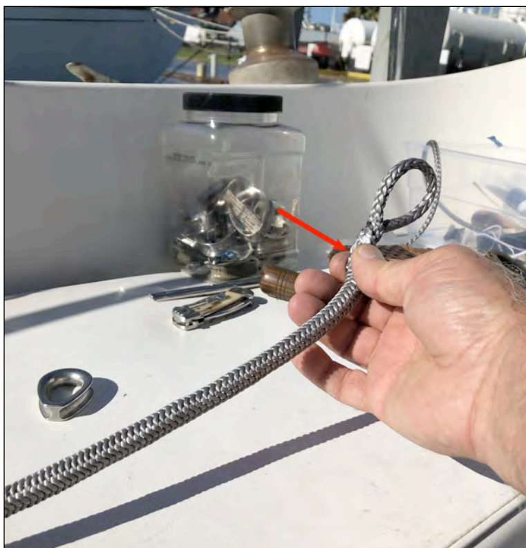
Step L - Pinch the Brummel cross over where the tail entered the body and only then pull the tail tight. Occasionally some gentle massaging of the pass through is necessary. Photo: Jamie White © 2020
