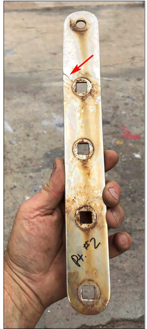
Port #2 chainplate. Note crack. Photo: Jamie White © 2020
