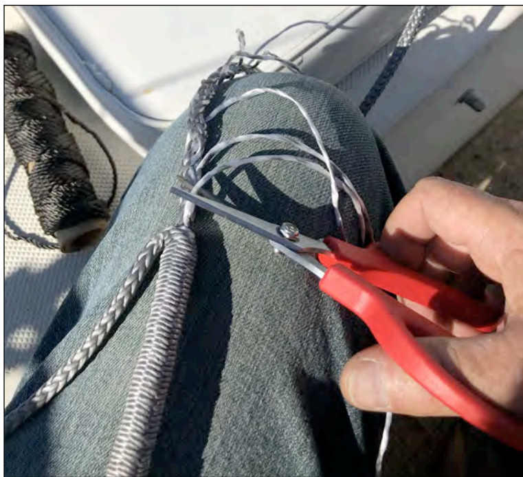
Step P - Trimming the pulled out yarns of the taper. I recommend a ceramic knife or serrated edge scissors designed to cut high-tech rope. I am using Ronstan splicing scissors from West Marine .
