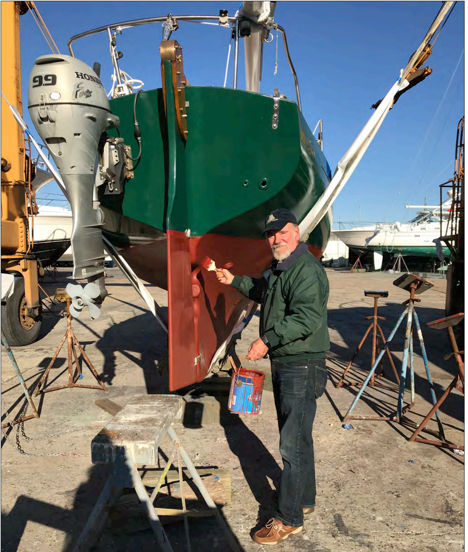
Final touch up of the bottom paint before launching. Note the refinished cheeks on the rudder.
