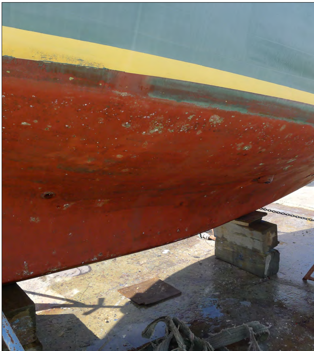
Topsides washed down and bottom pressure washed. I was surprised just how much bottom paint was intact after over 10 years since last haul-out. Photo: Jamie White © 2020
