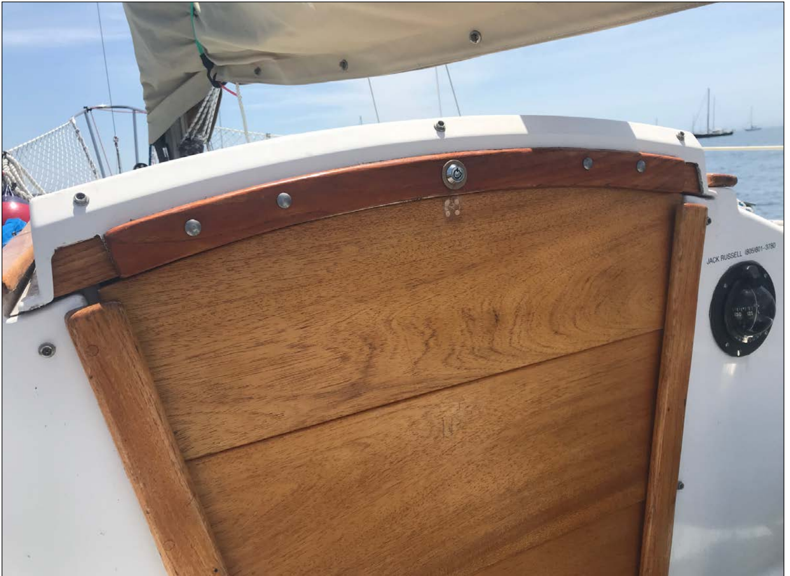
The completed project to fill the gaps and upgrade the lock on the companionway slide. Photo: Jack Russell © 2020
