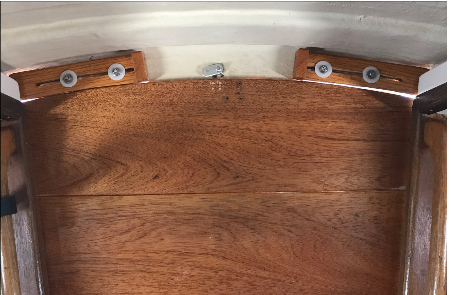
Port and starboard slides in place. Note the barrel bolt that replaces the original hasp. Photo: Jack Russell © 2020
