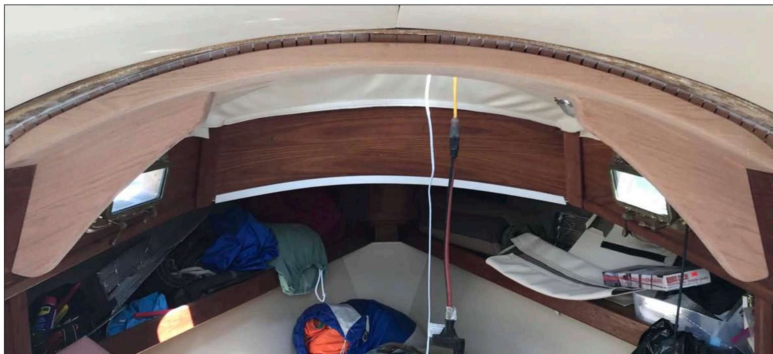
The faceplate curves on the fore and aft were easy to pattern and that is what made the arch super strong! A few nails and glue there too. The faceplate only covers the first two arch boards leaving a space for antenna and mast light wires and a place for the ceiling panels to lay on top. Photo: Jack Russell © 2020
