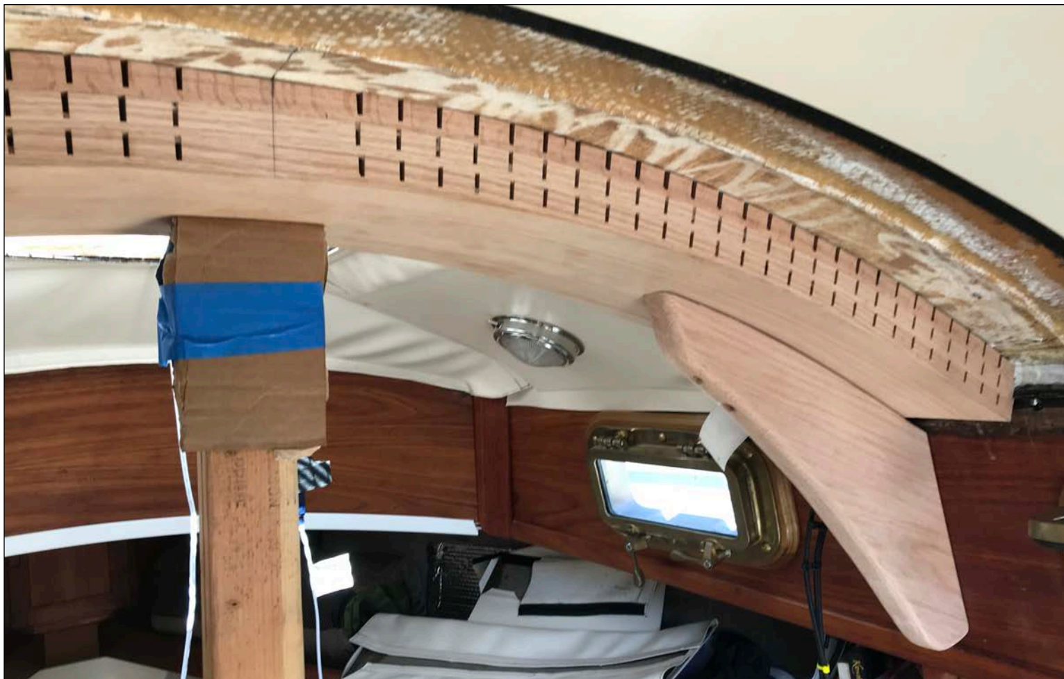
Building the knee supports turned out to be the most difficult part. There are so many darn angles to account for! Again, with a lot of cardboard patterns using trial and error. They are bolted to the side walls with stainless steel lags and fender washers from the outside. Photo: Jack Russell © 2020
