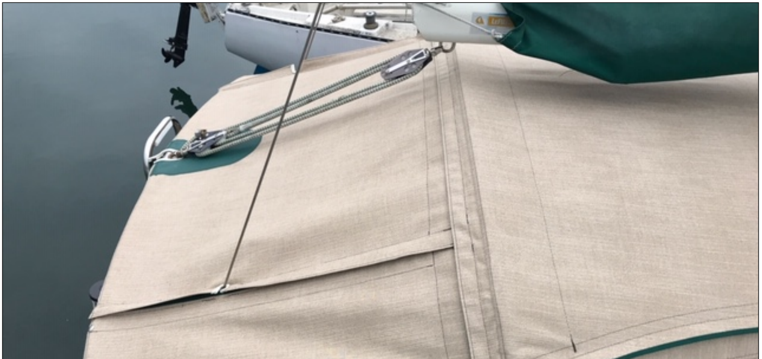
Aft panel of the cockpit enclosure. Note the precise placement of the aft split stay wire in the panel. Photo: Tim Wild © 2020
