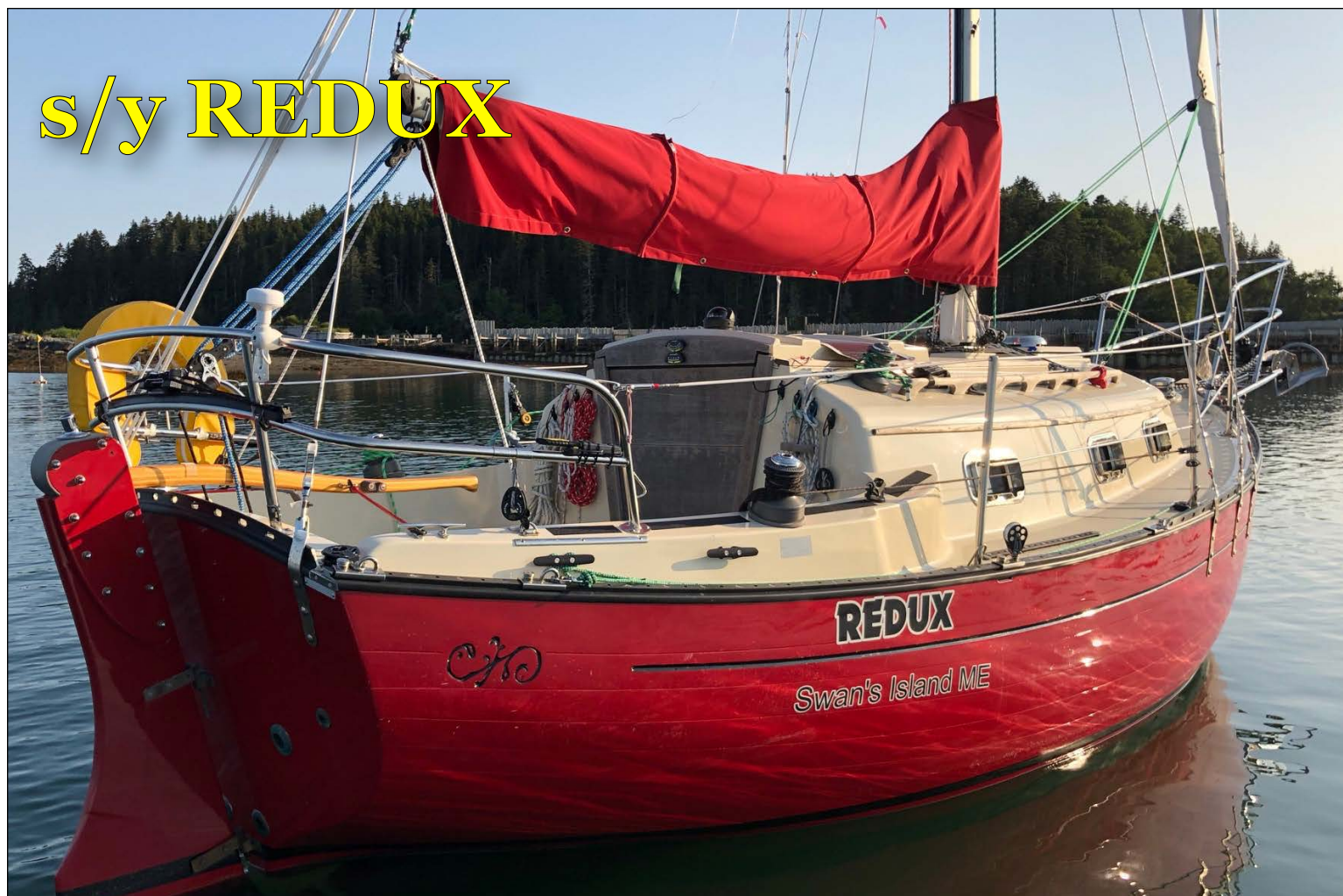
REDUX riding on her mooring in Burnt Coat Harbor. Note the traveler on the stern pulpit. Rigged for self-tacking using the green sheets on the jib. Photo: Jay Cushman © 2020
