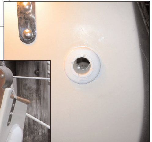
The vent emerges through the transom near the top. A marelon thru-hull and clamshell vent cover complete the installation.
